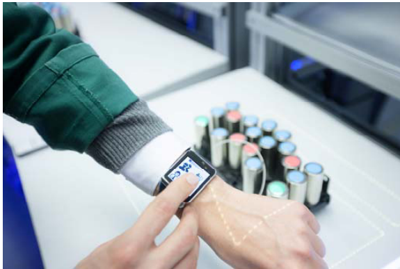
Fig. 3. Smart watch with the button to call for an expert
