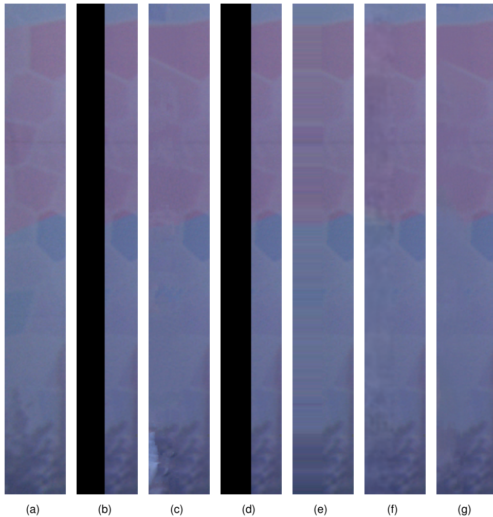
Figure 4.11.: Inpainting results from different inpainting algorithms for the left border of test image 3. From left to right: reference image, image with hole, Criminisi, Gautier, VSRS, MS-KSVD-D, MS-SSD-D.
