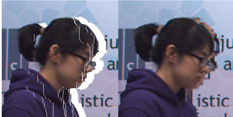
Figure 2.21.: Problem occurring during inpainting process with Criminisi et al. [1]. Hole (in white in the left image) associated to the background is partly inpainted on the right image with texture information from the person in the foreground.
