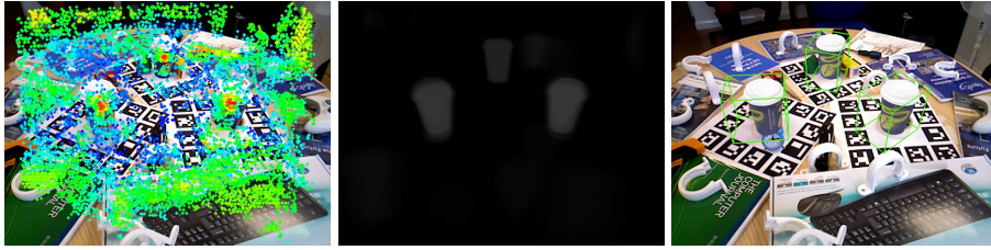
Figure 4.3: Example of detection of multiple objects in a RGBd image. On the left, the representation of vote accumulation (red means high number of votes), in the center approximate segmentation resulting from the back-projection of votes and patch-masks scaled by the vote weight, on the right detection result with pose.
