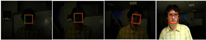
Figure 5.5: Robustness towards illumination changes is achieved by normalizing the patches extracted from the image. Even in sequences like 'David', where extreme illumination changes are present, our method performs correctly.
