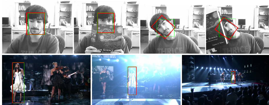
Figure 5.3: Our method, whose output is depicted using a red bounding box, is able to cope with large rotations and scale changes. Note that the manual annotation provided in the benchmark data-set [172], depicted in green, does not take into account rotations.
