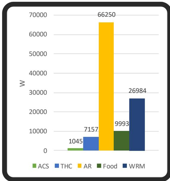
Figure 10-37: Power requirements of the different subsystem for Case4 in a recycling system
