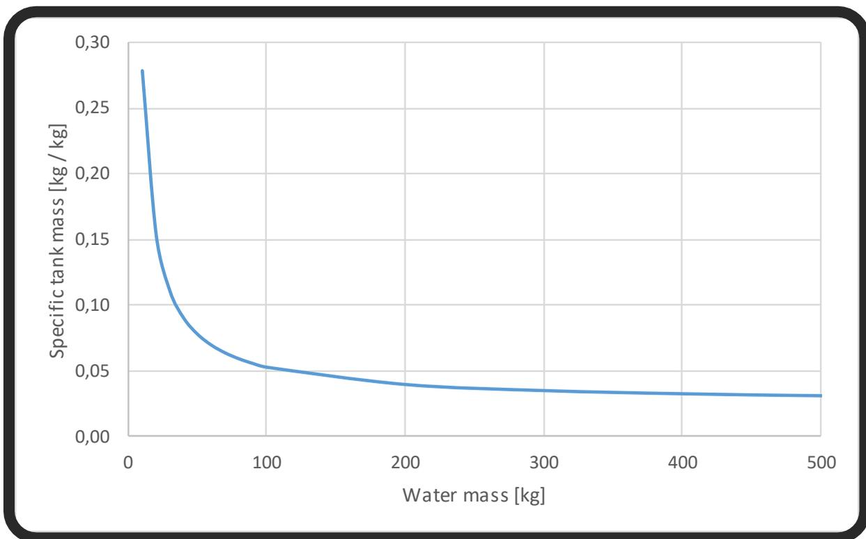
Figure 6-23: Specific water tank mass for water masses up to 5,000 L
