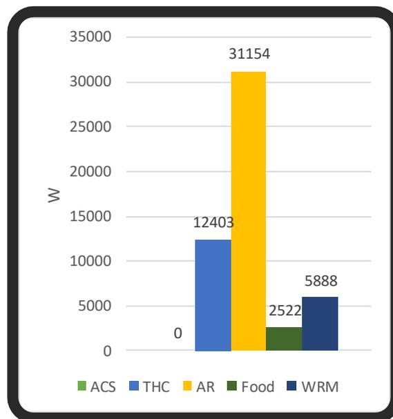
Figure 10-30: Cooling requirements of the different subsystems for Case2
