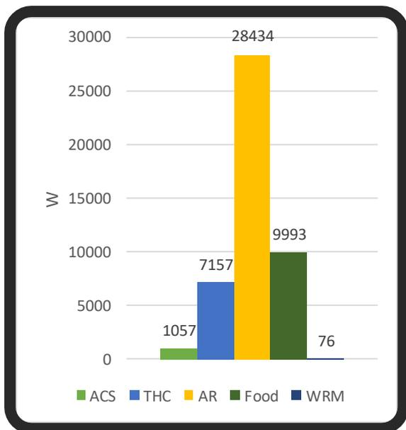
Figure 10-41: Power requirements of the different subsystems for Case4 in a storage system
