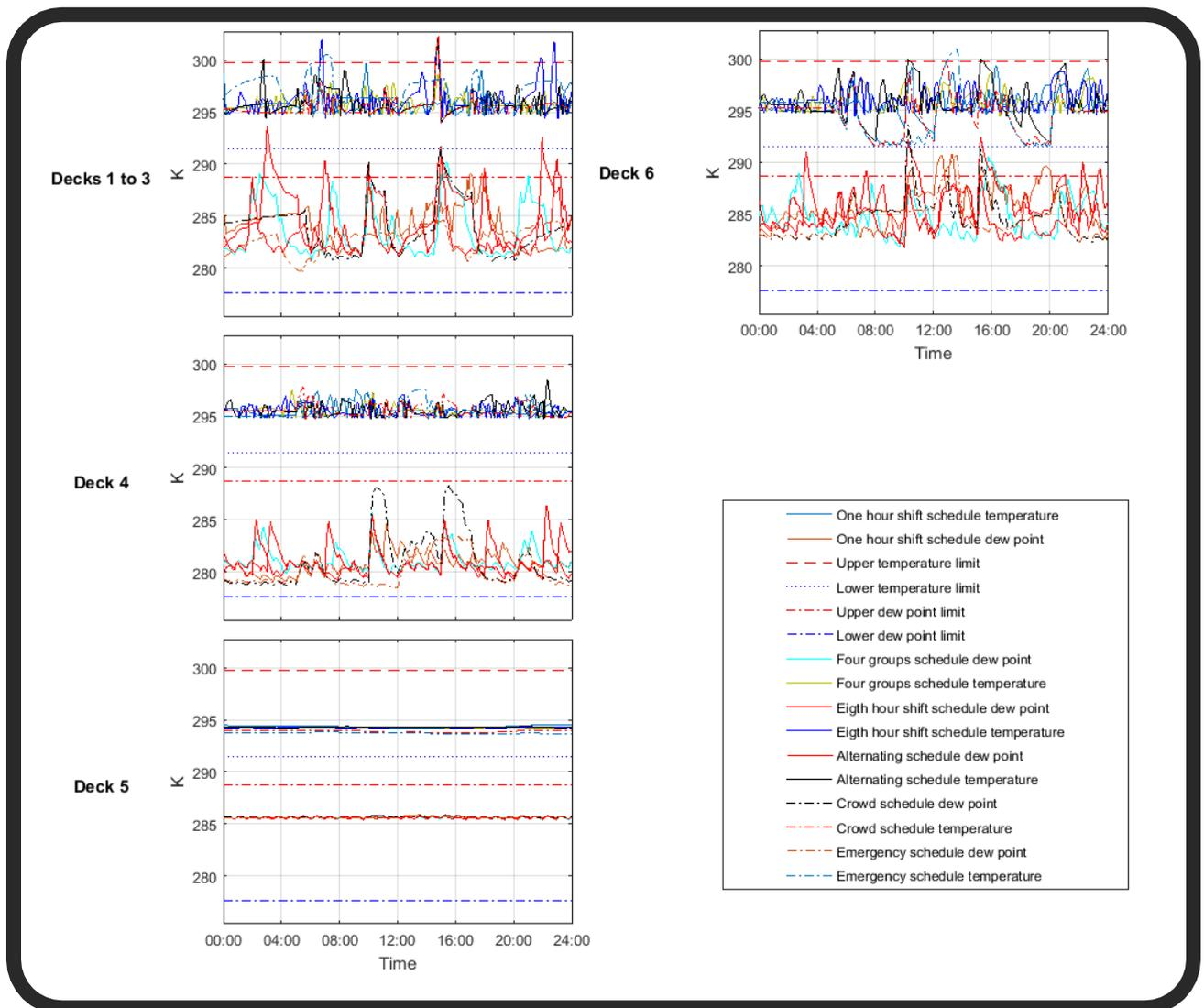
Figure 11-17: Comparison plot of temperature and dew point between the schedules
