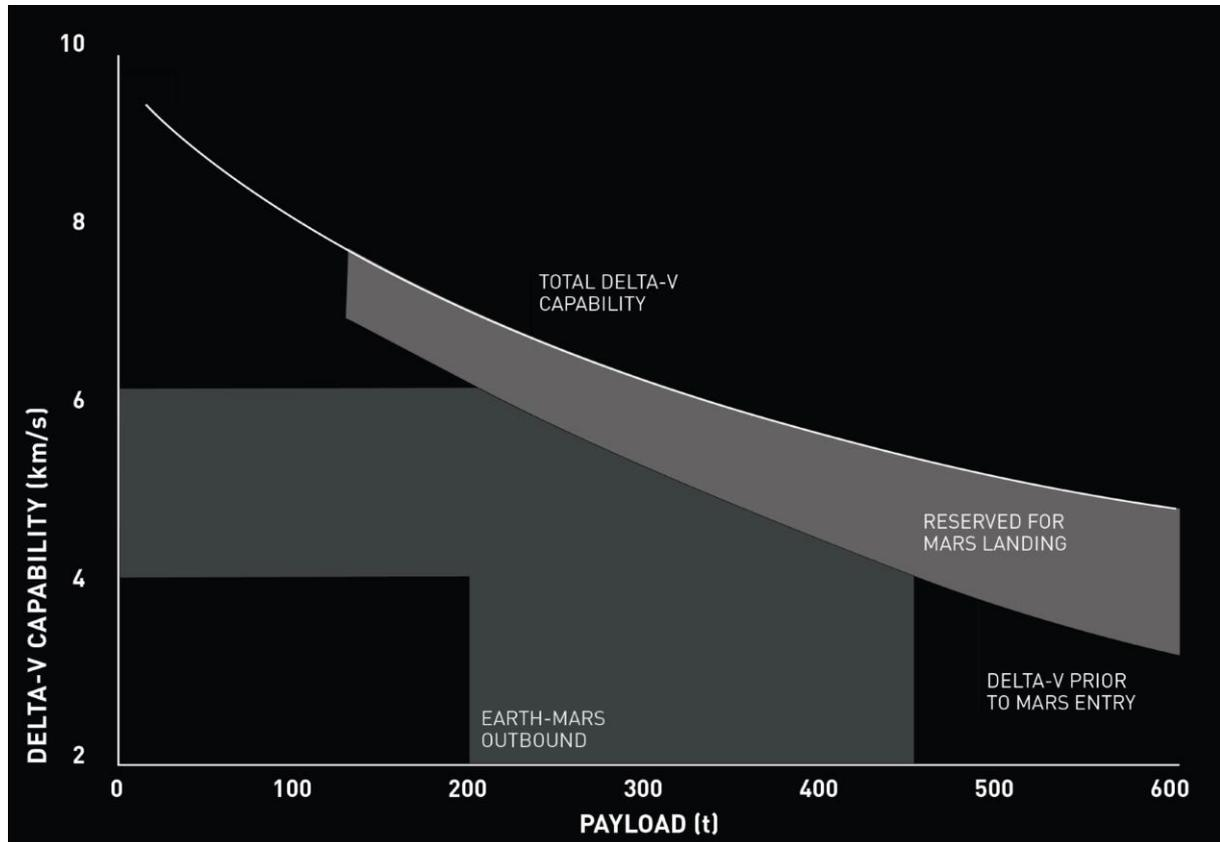
Figure 2-4: SpaceHab  $\Delta v$  and Payload capacity [1]
