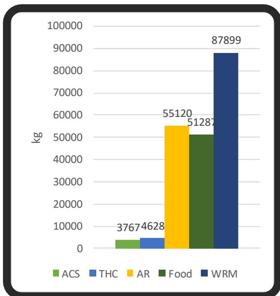
Figure 10-35: Mass of the different subsystems for Case4 in a recycling system
