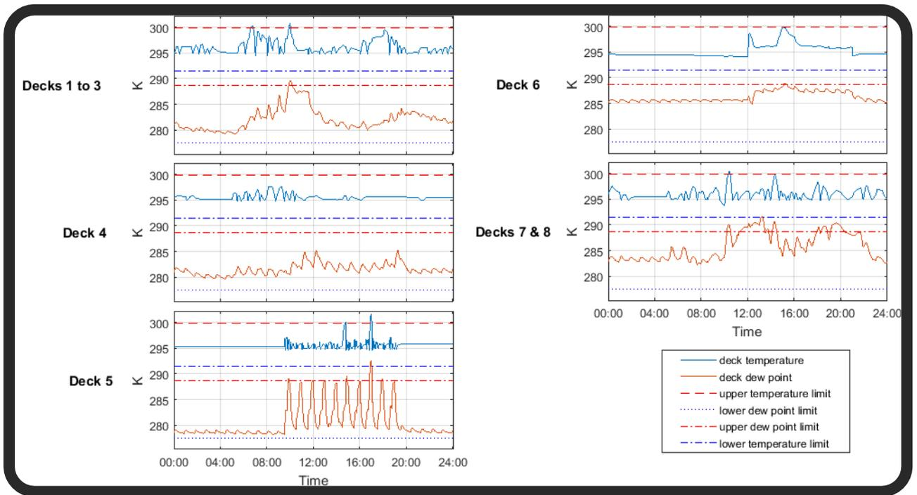
Figure 11-14: Verification plot of the temperature and dew point for Evolved-SpaceHab, 100 passengers, and one hour shift schedule over one day
