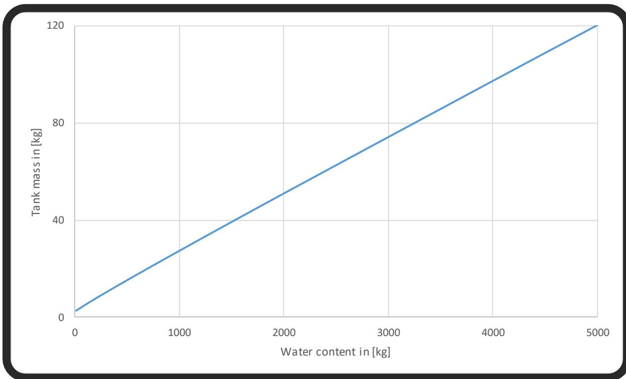
Figure 6-22: Bladder tank mass for water masses between 10 and 5,000 kg.
