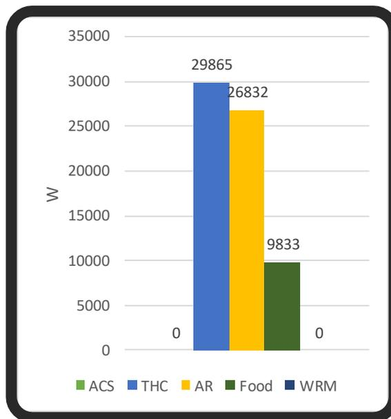
Figure 10-42: Cooling requirements of the different subsystems for Case4 in a storage system
