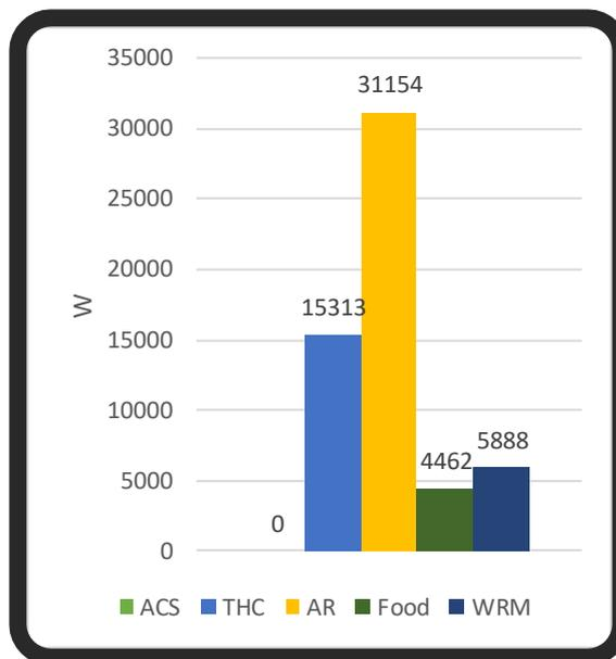
Figure 10-34: Cooling requirements of the different subsystems for Case3
