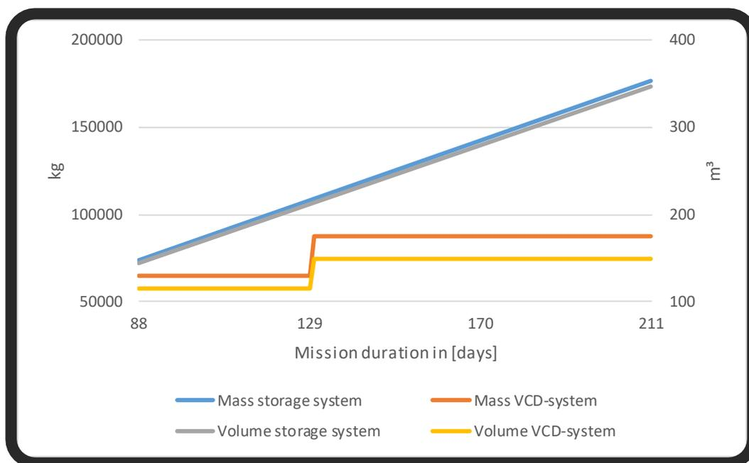
Figure 10-20: Required mass and volume for a storage and recycling water system over time for 100 people
