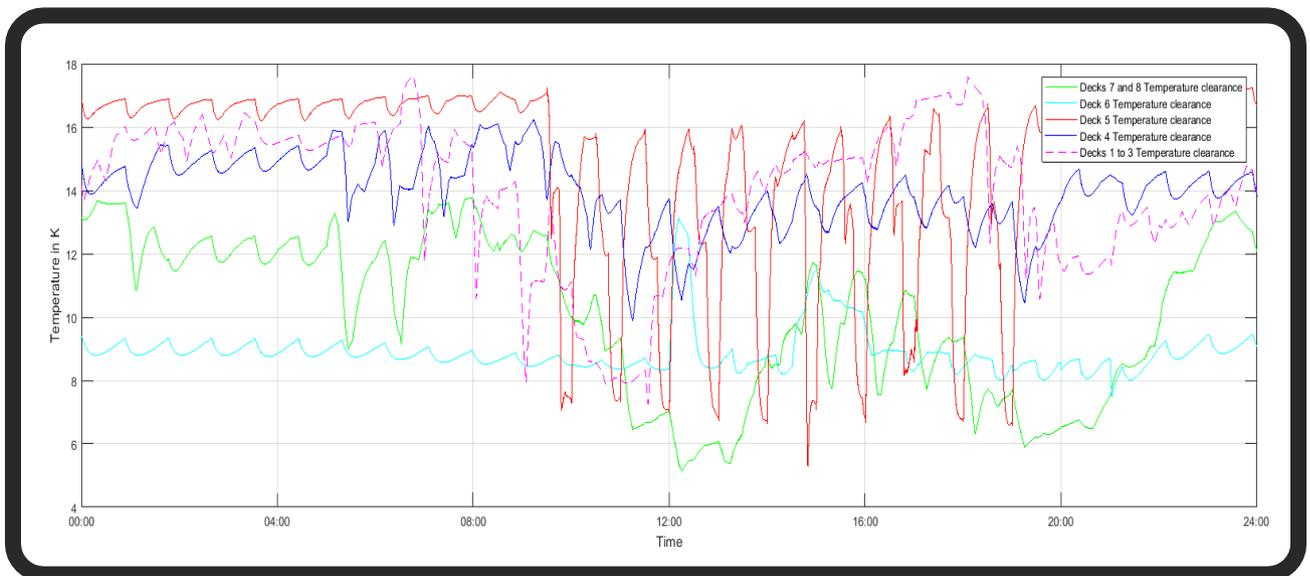
Figure 11-15: Clearance between dew point and temperature for Evolved-SpaceHab, 100 passengers, and one hour shift schedule over one day
