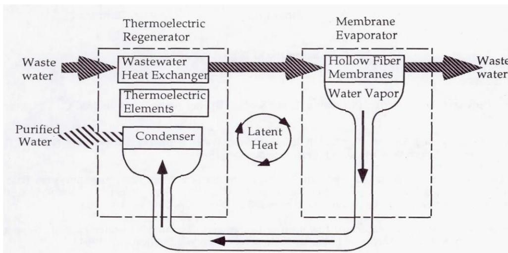
Figure 6-30: TIMES schematic [55, p. 230]
