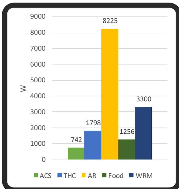
Figure 10-25: Power requirements of the different subsystem for Case1
