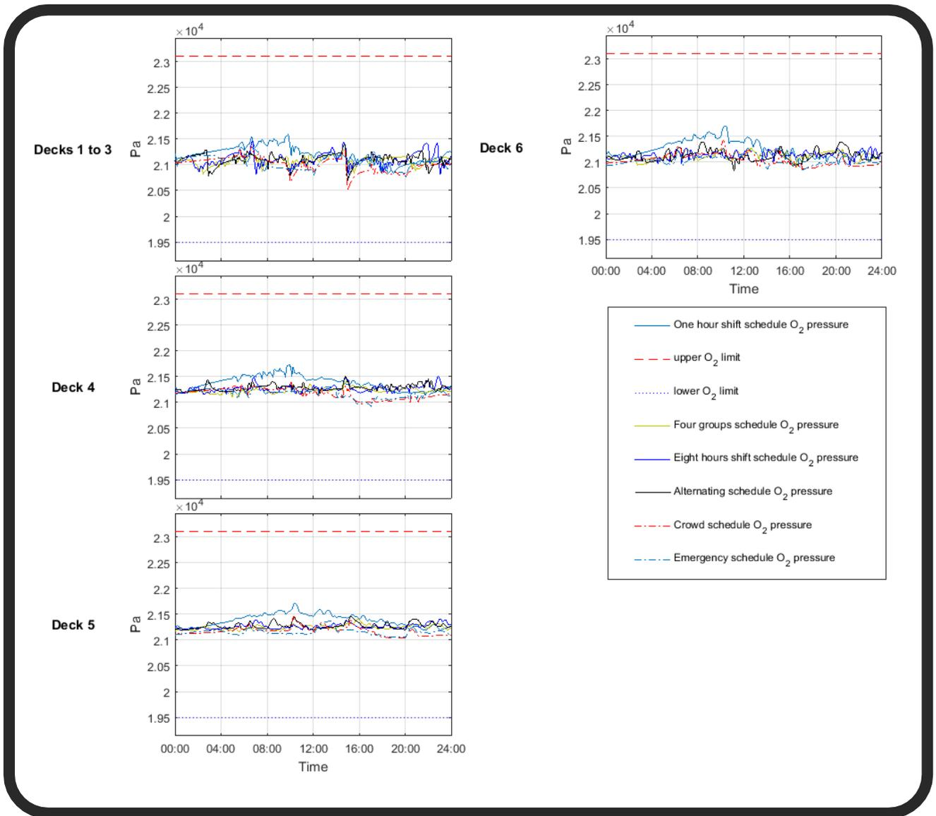
Figure 11-19: Comparison plot of partial O<sub>2</sub> pressure between the schedules
