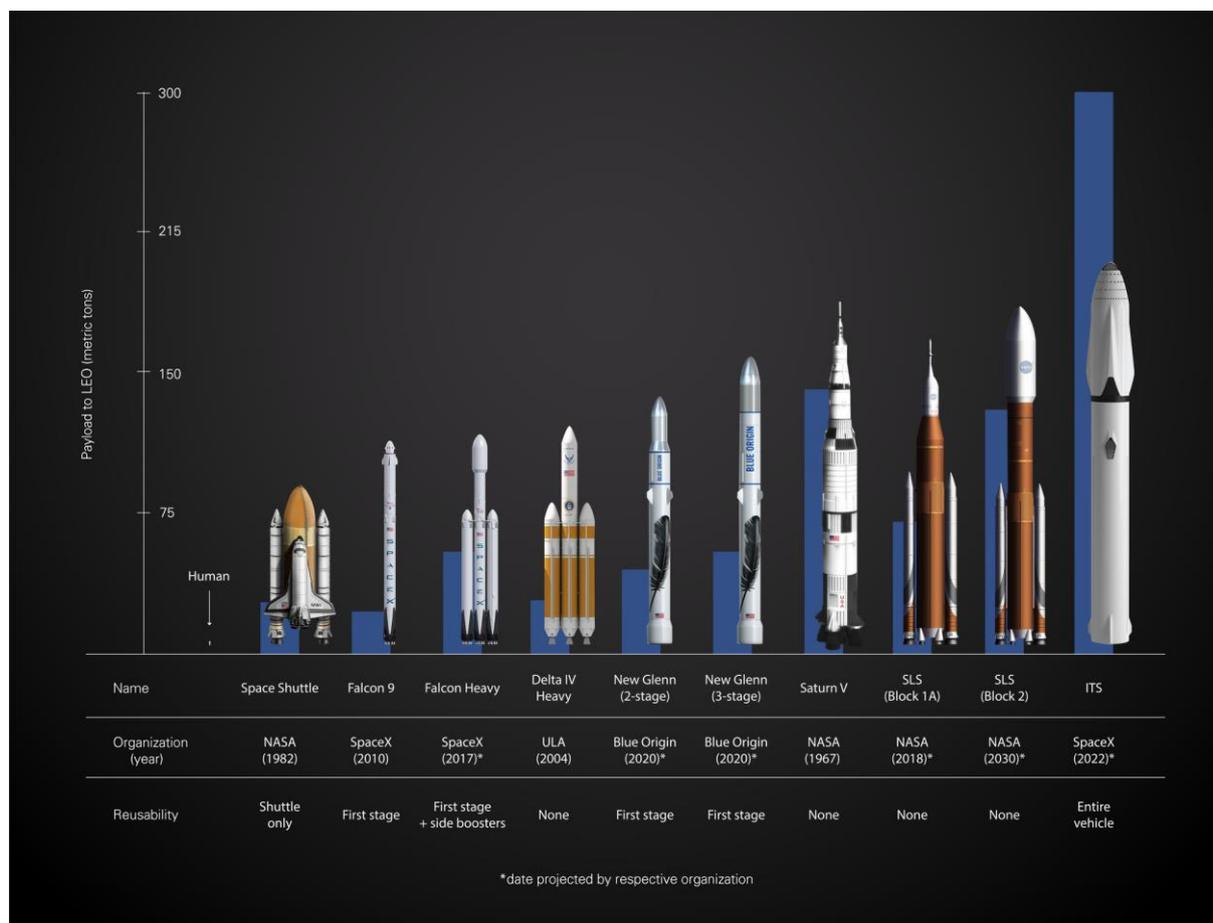
Figure 2-1: Comparison of ITS (right) with other Rockets [12]
