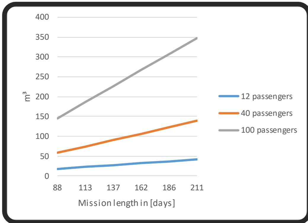
Figure 6-24: Required volume for the water storage system depending on mission length and crew size
