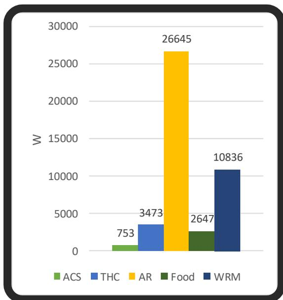
Figure 10-29: Power requirements of the different subsystem for Case2
