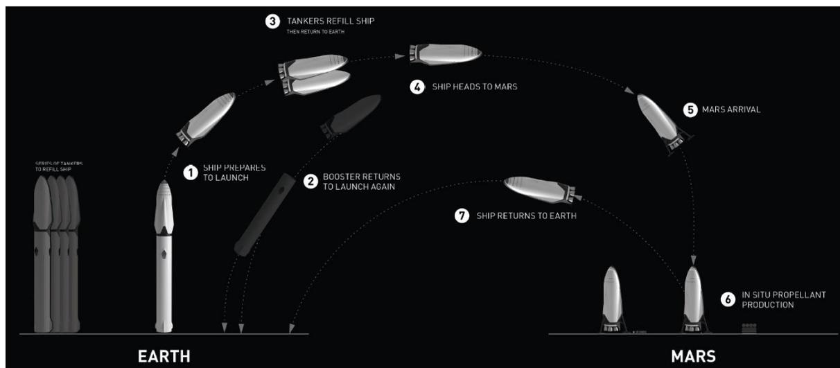
Figure 3-1: Proposed high-level operations profile by SpaceX [1]
