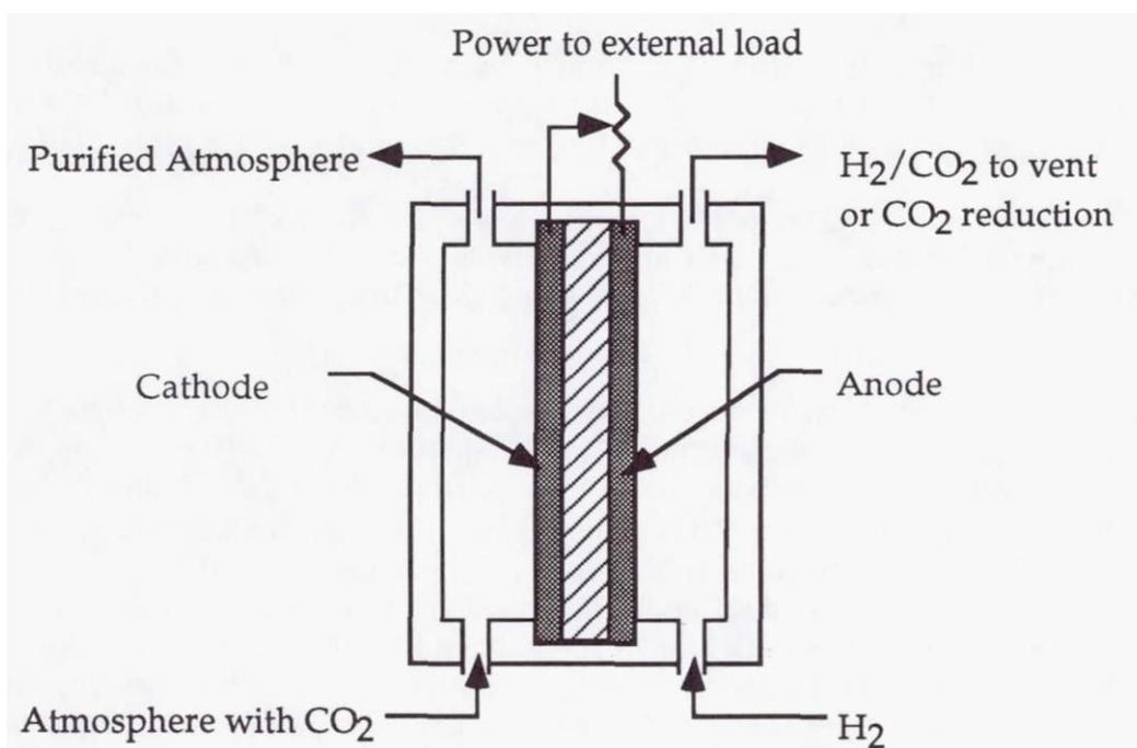
Figure 6-15: EDC schematic [55, p. 193]
