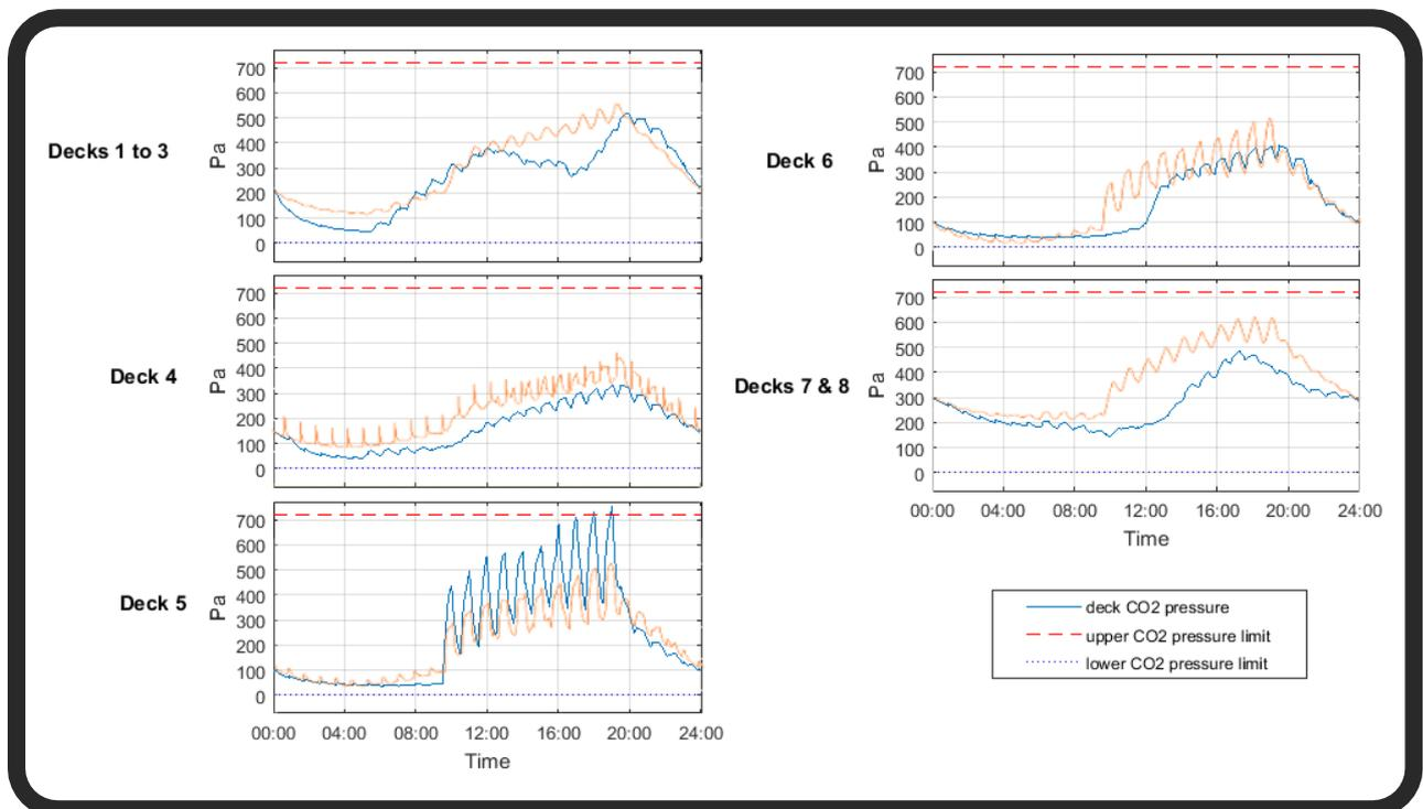
Figure 11-12: Verification plot of the partial carbon dioxide pressure for Evolved-SpaceHab, 100 passengers, and one hour shift schedule over one day
