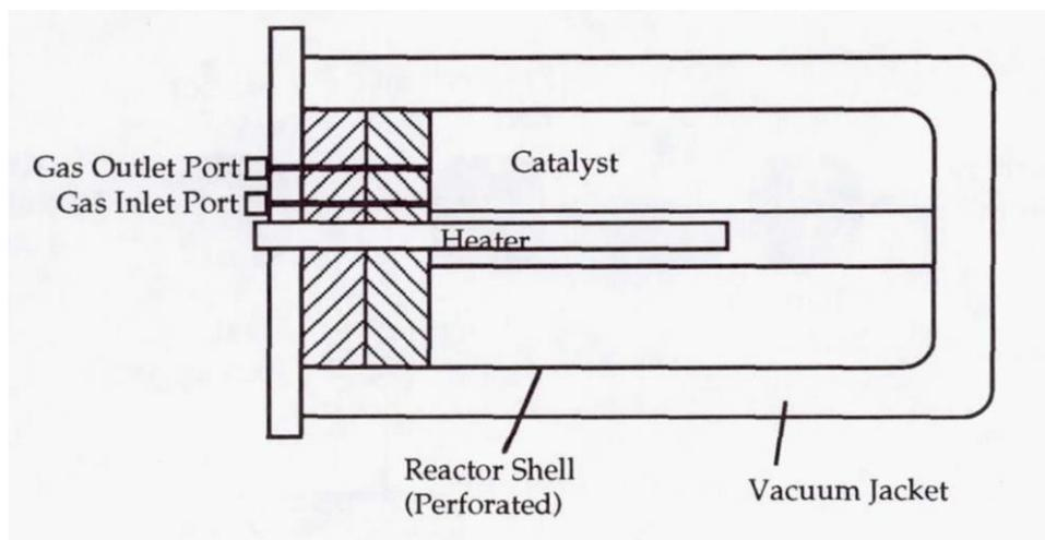
Figure 6-17: Bosch reactor [55, p. 199]
