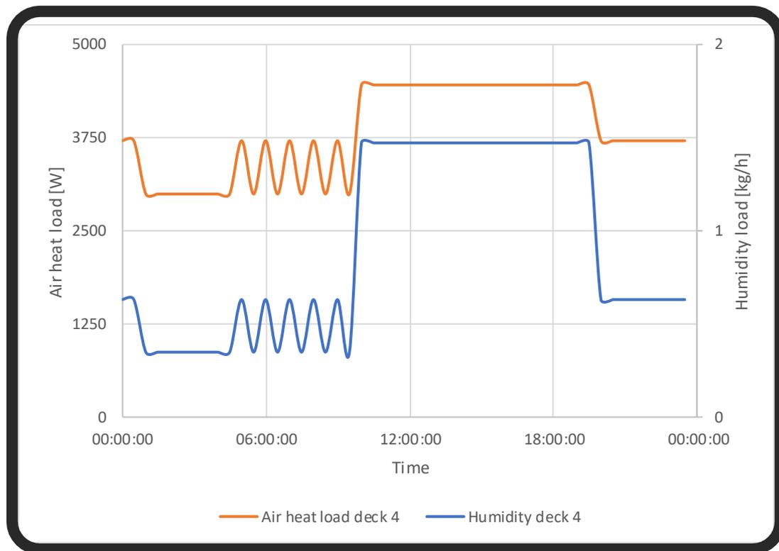
Figure 10-11: Air heat and humidity loads over 24 hours in deck 4 with 100 passengers and the one hour schedule
