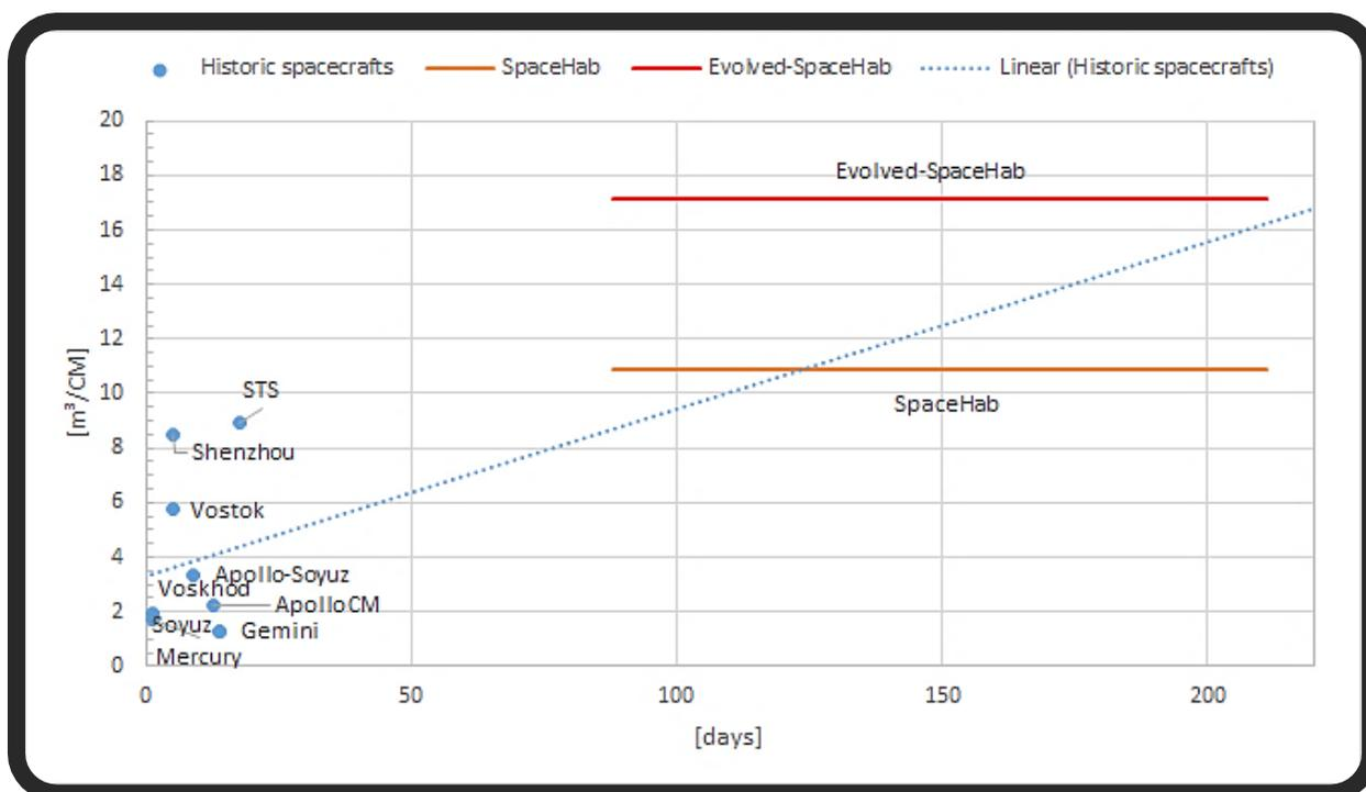
Figure 3-4: Plot of pressurized volume per CM for historic spacecraft's and the considered SpaceHab designs with 100 CM
