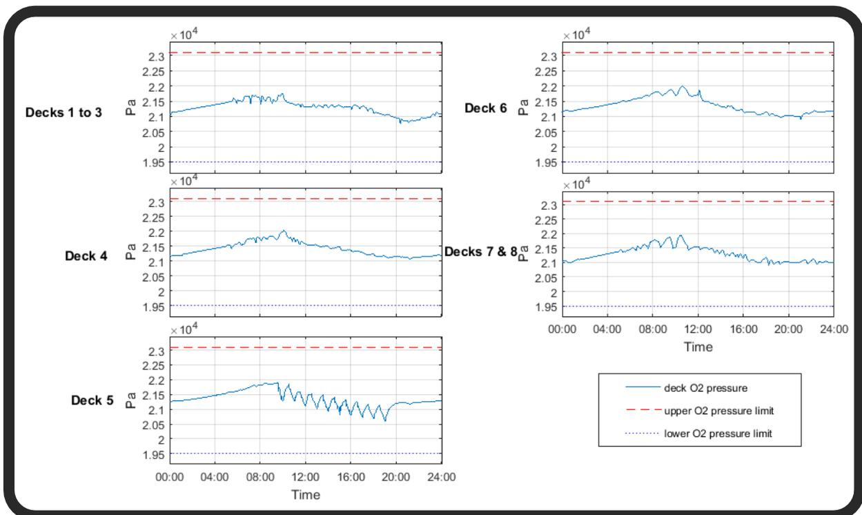
Figure 11-11: Verification plot of the partial oxygen pressure for Evolved-SpaceHab, 100 passengers, and one hour shift schedule over one day
