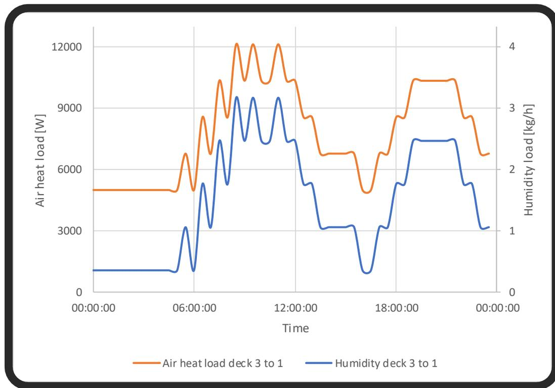
Figure 10-13: Air heat and humidity loads over 24 hours in decks 1 to 3 with 100 passengers and the one hour schedule
