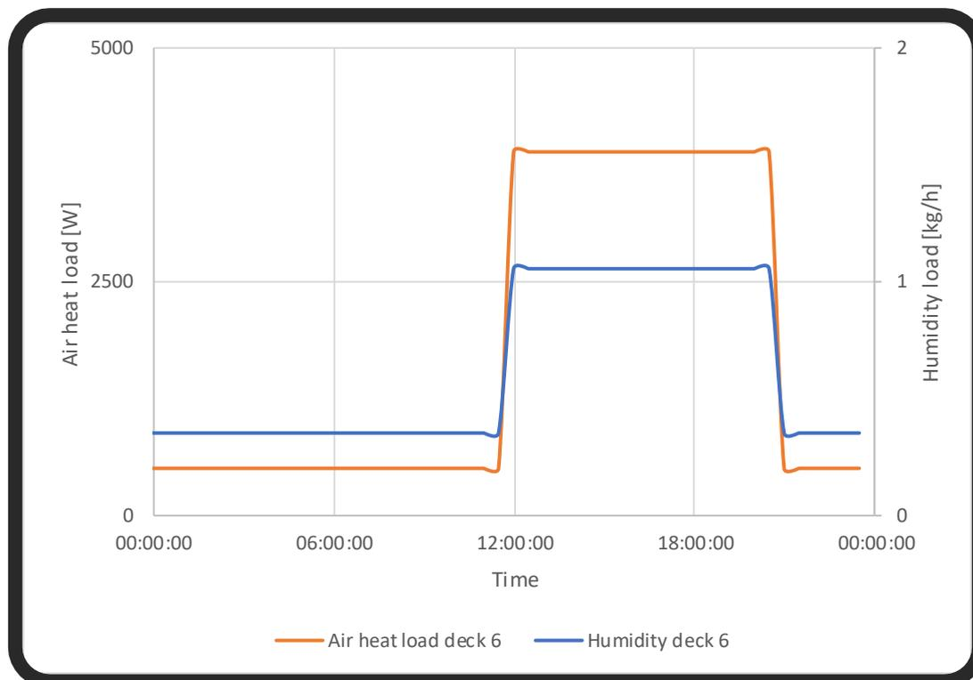
Figure 10-7: Air heat and humidity loads over 24 hours in deck 6 with 100 passengers and the one hour schedule
