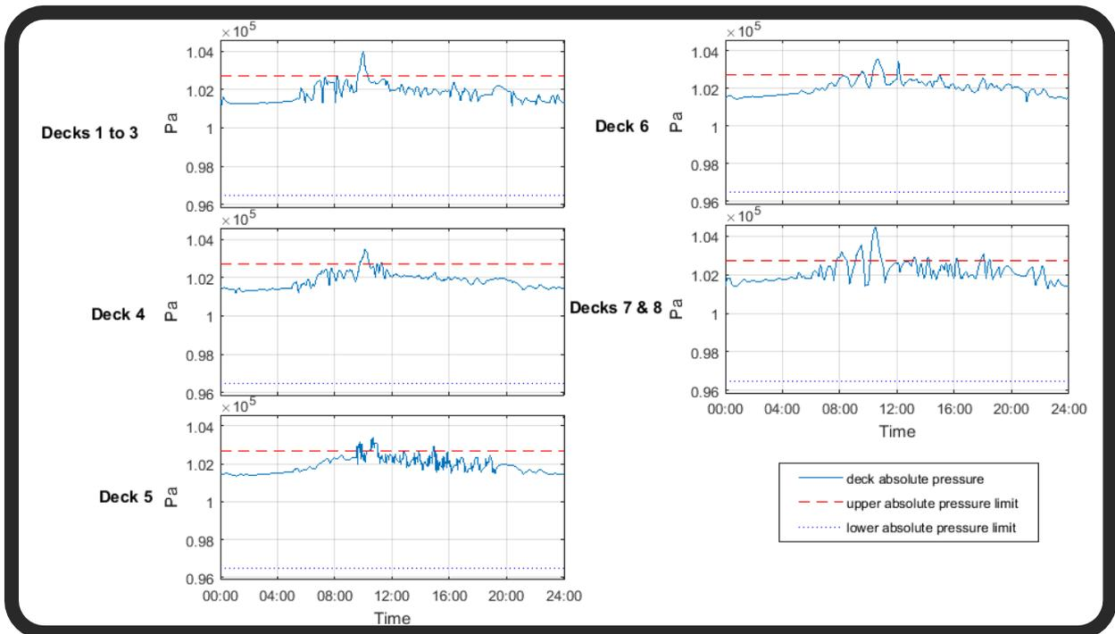
Figure 11-10: Verification plot of the total pressure for Evolved-SpaceHab, 100 passengers, and one hour shift schedule over one day
