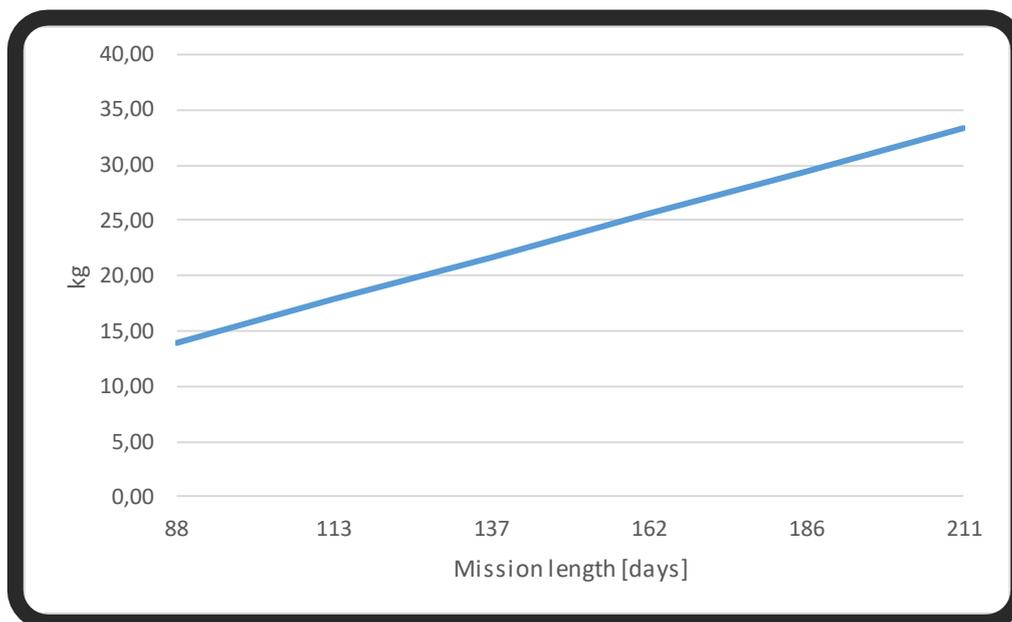
Figure 4-2: N<sub>2</sub> leakage mass over mission length
