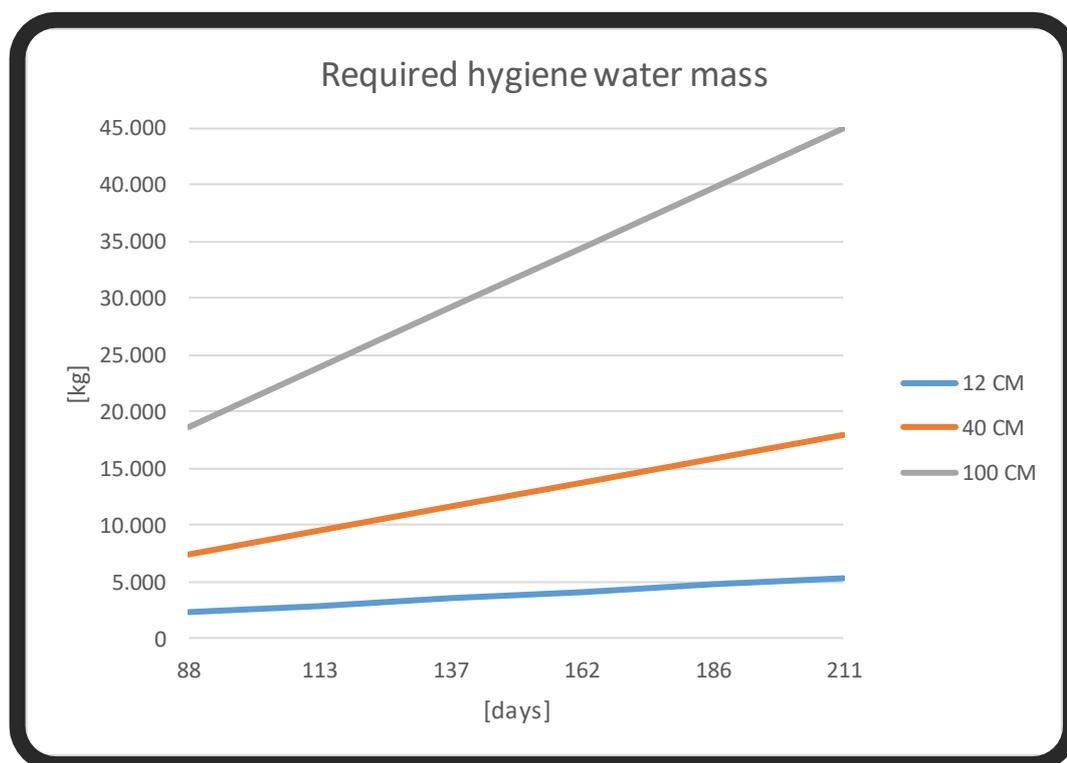
Figure 4-5: Required hygiene water mass of a storage system for the considered scenarios
