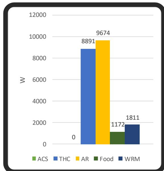
Figure 10-26: Cooling requirements of the different subsystems for Case1
