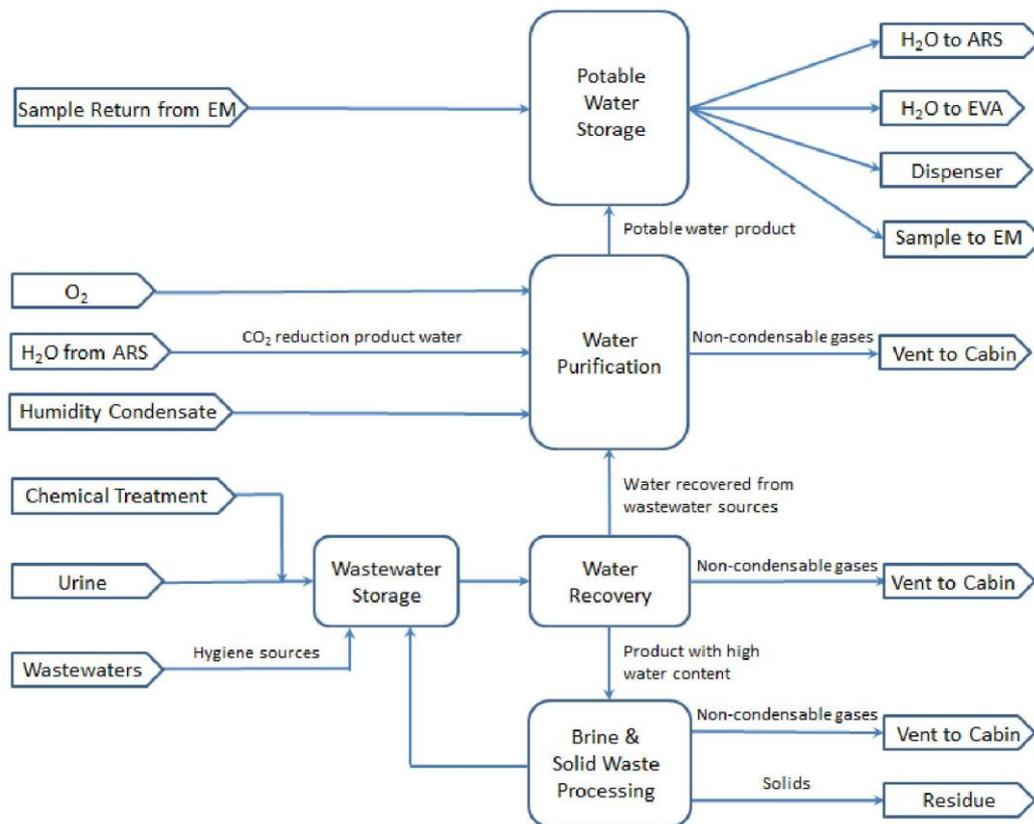
Figure 6-20: WRM schematic [17, p. 7]
