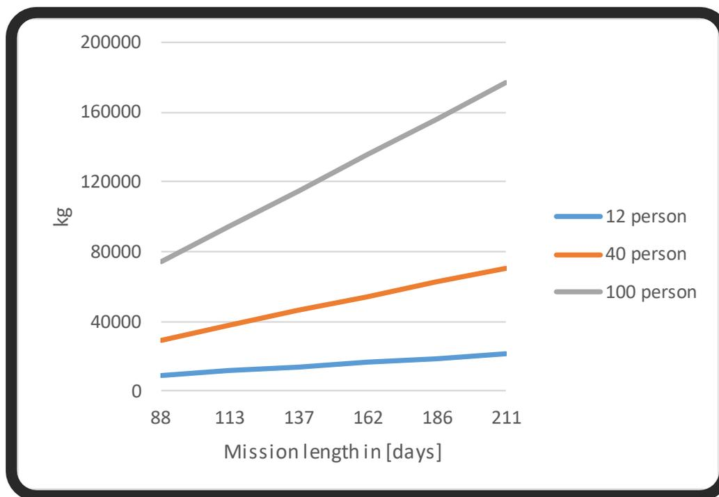
Figure 6-25: Required mass for the water storage system including potable water mass depending on mission length and crew size
