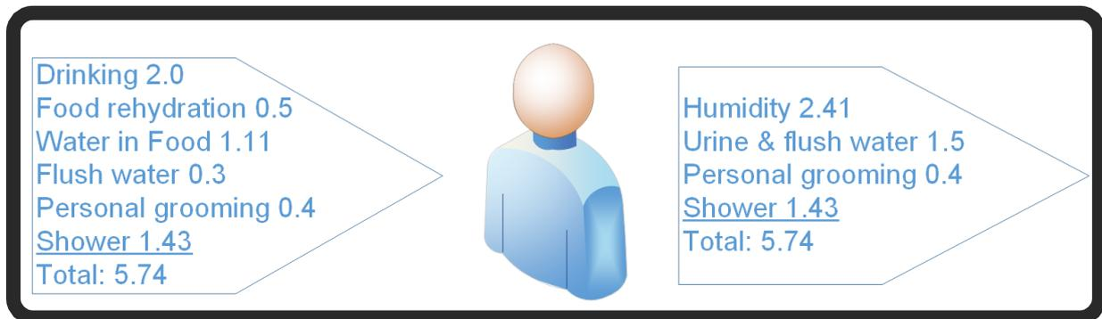
Figure 6-21: Water balance in [kg CM-d<sup>-1</sup>]
