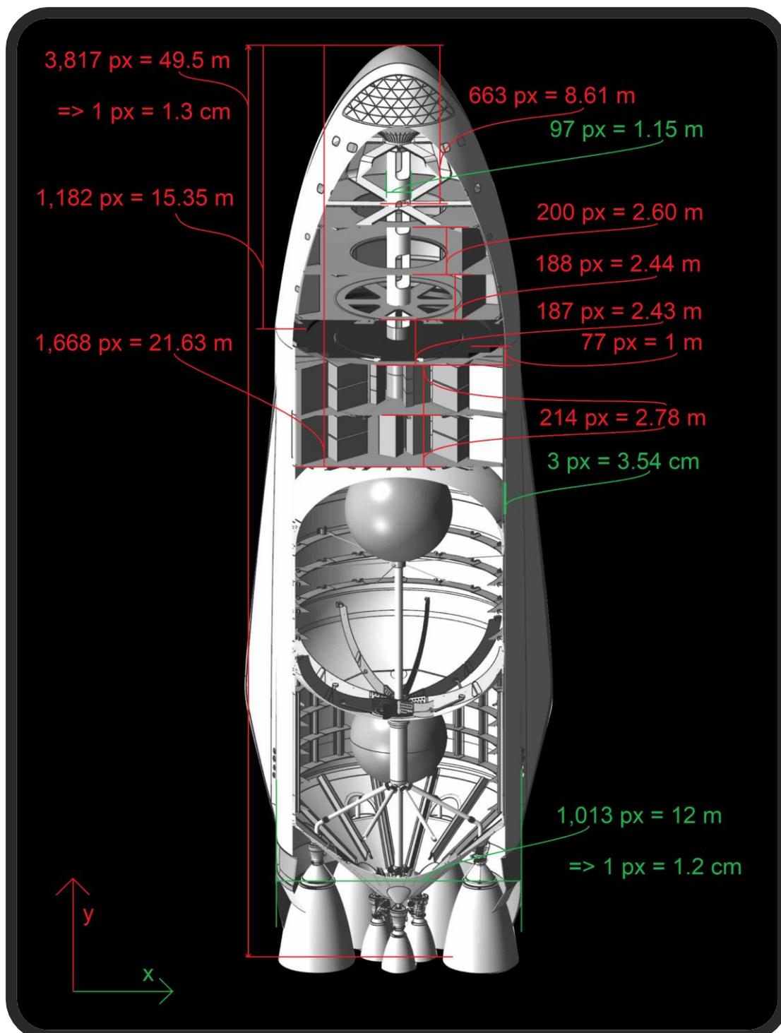
Figure 2-2: Spaceship dimensions [SpaceHab picture from [1]]
