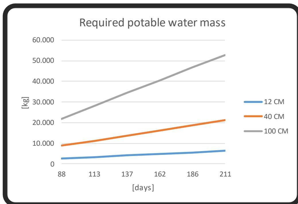
Figure 4-4: Required potable water mass of a storage system for the considered scenarios
