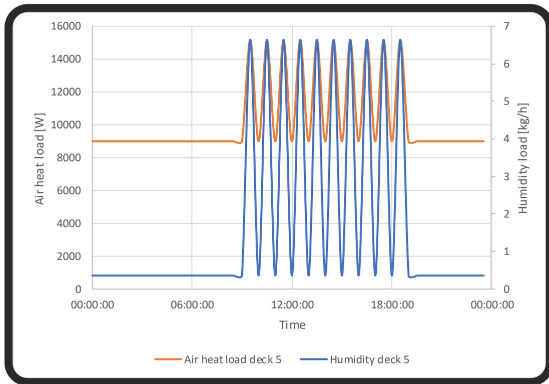
Figure 10-9: Air heat and humidity loads over 24 hours in deck 5 with 100 passengers and the one hour schedule
