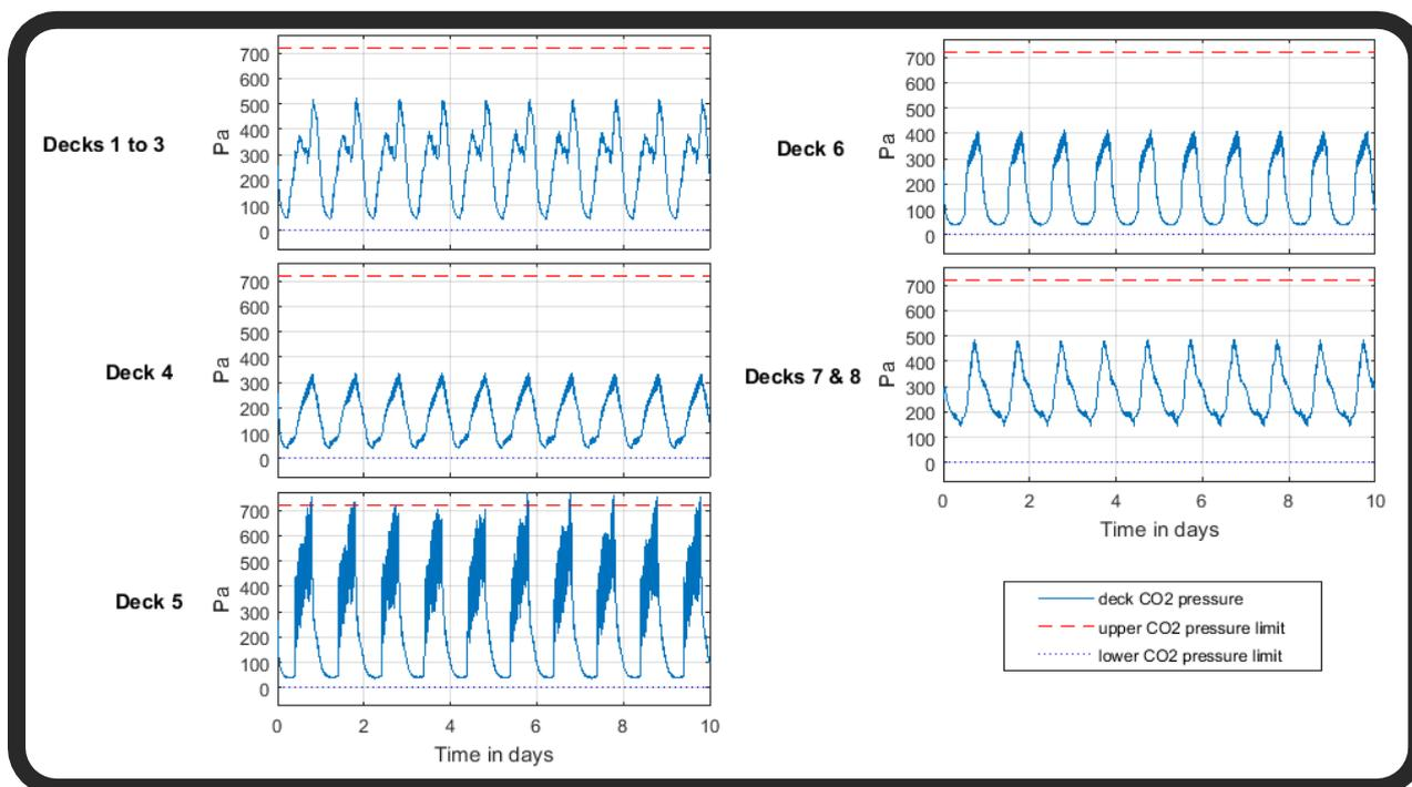
Figure 11-13: Verification plot of the partial carbon dioxide pressure for Evolved-SpaceHab, 100 passengers, and one hour shift schedule over ten days
