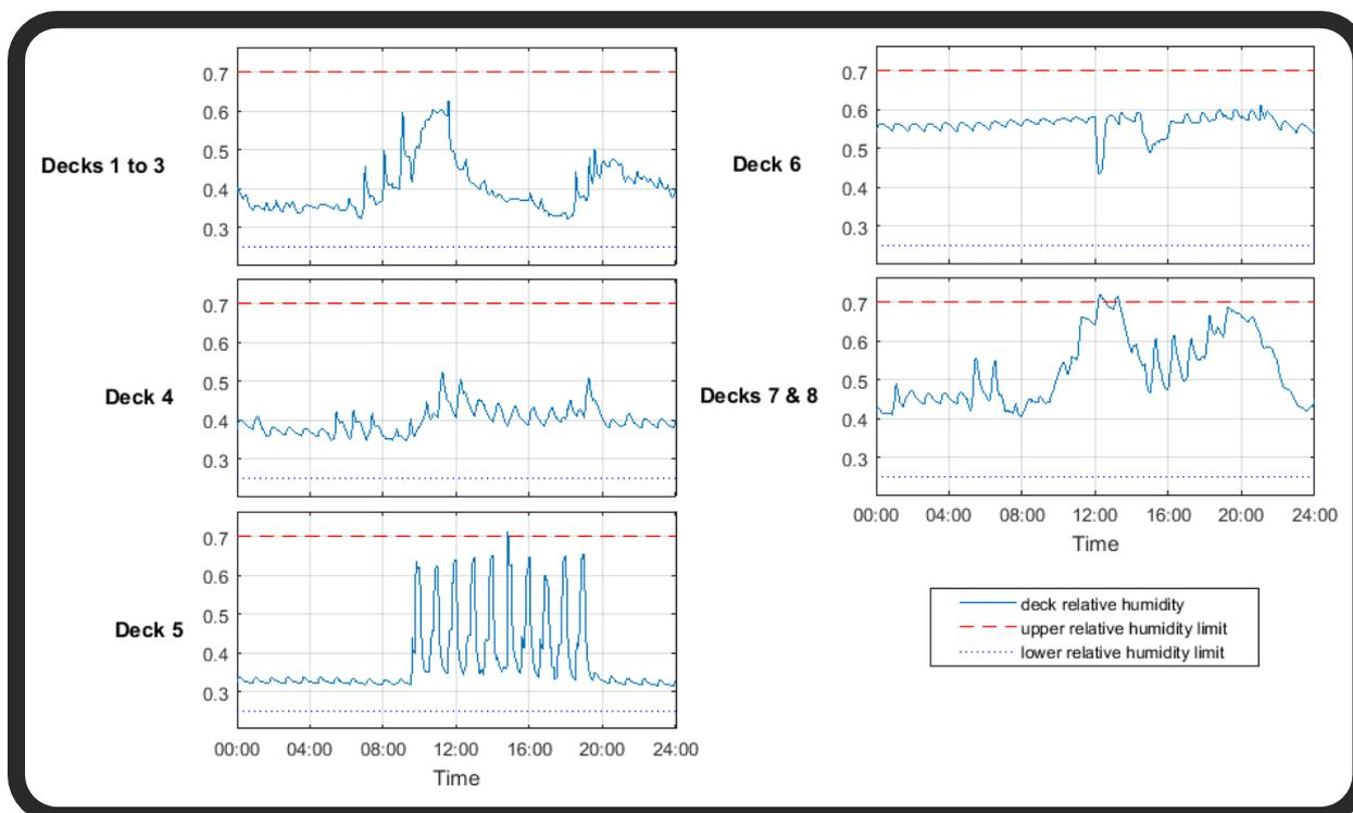
Figure 11-16: Verification plot of the relative humidity for Evolved-SpaceHab, 100 passengers, and one hour shift schedule over one day
