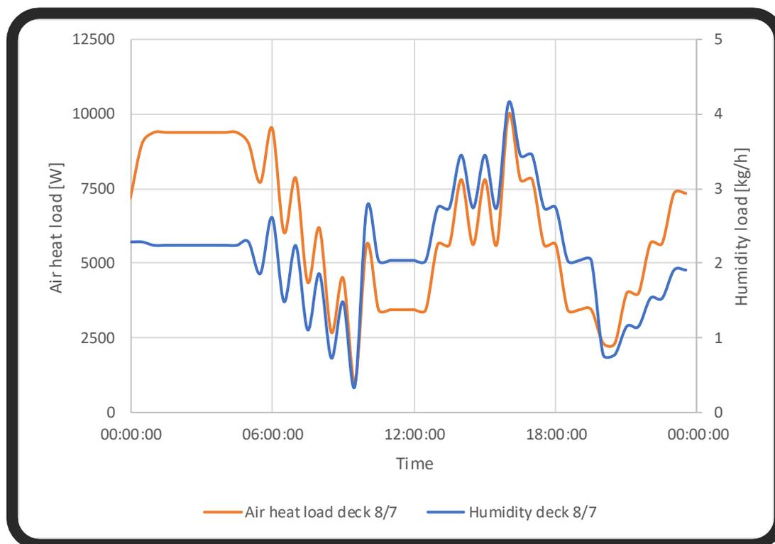
Figure 10-4: Air heat and humidity loads over 24 hours in decks 7 and 8 with 100 passengers and the one hour schedule
