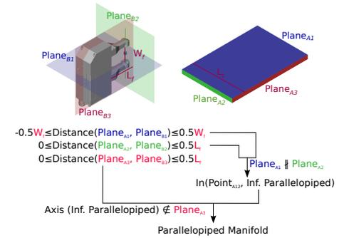
Fig. 5: Constraint combination rules for a task with inequality constraints (tray grasping)
