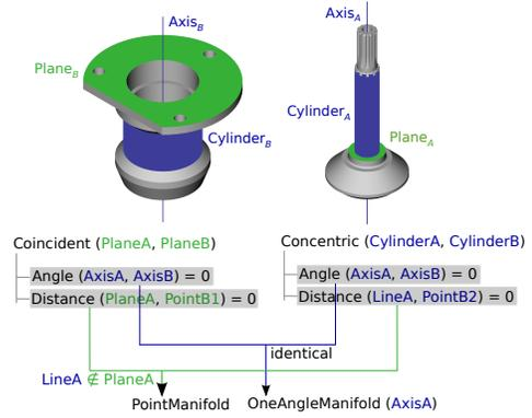
Fig. 4: Example of constraint combination rules for assembly.
