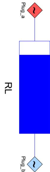
The model contains equations for harmonic domain and ABC system. All relationships which are common by **two-port elements** (R,L,C,...) are shifted to the sub-model “TwoplugPhasor”.
