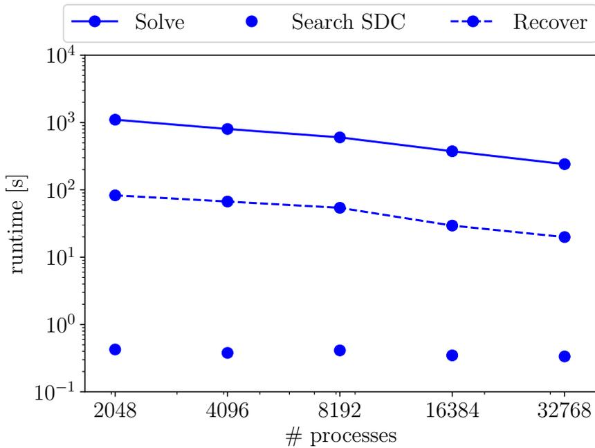
**Figure 6.15:** Scaling experiments with SDC detection on. We used 8 process groups and varied the number of processes per group, doubling from 256 until 4096. The total computational time required to ensure silent error resilience (*Search SDC* + *Recover*) is still one order of magnitude smaller than one single time step of the PDE solver (As submitted in [PHBP].)
