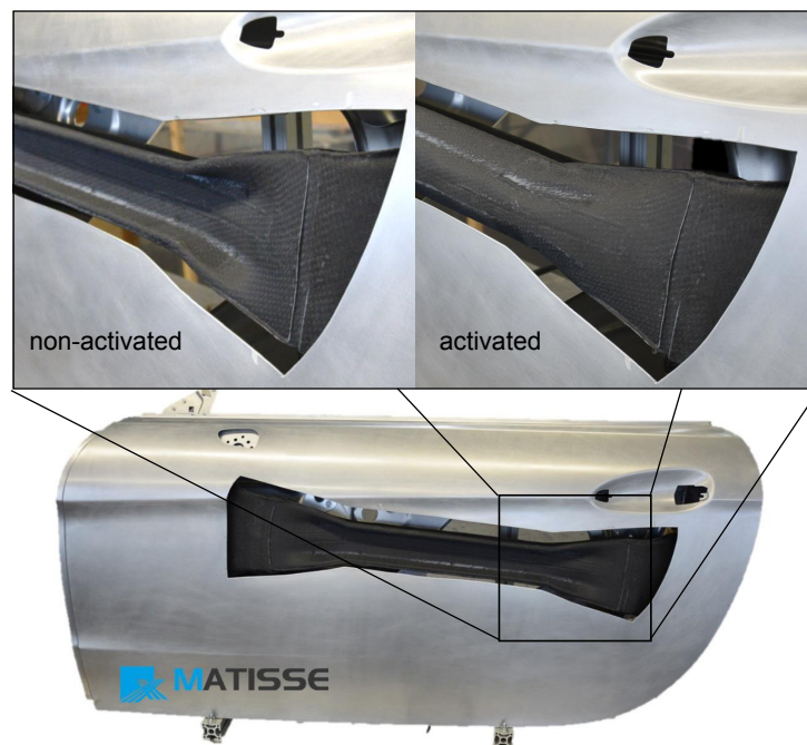
Figure C-2 Shape adaptive CFRP crash structure in hybrid-matrix design: non-activated and activated
