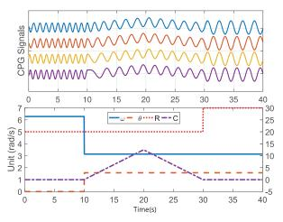
Fig. 6: CPG output waves with changing parameters controlled by high-level brain model. The upper figure shows four CPG output signals. The bottom figure shows different sets of CPG parameters.
