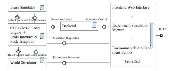
Fig. 4: Functional architecture of the NRP consisting of 6 key software components: Brain Simulator, World Simulator, Brain Interface and Body Integrator, Closed Loop Engine, Backbend, and Frontend.
