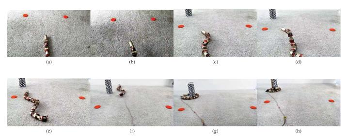
Fig. 8: Montage of the snake-like robot achieves semi-autonomous locomotion. The orange pads are used as the reference positions.
