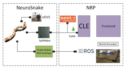
Fig. 2: A hybrid simulation and neuromorphic computing paradigm by combining the Neurorobotics Platform (NRP) [4] and the neuromorphic snake-like robot *the NeuroSnake*. ROS interface connects them to each other. SpiNNaker is able to be integrated into the close loop experiments. For the details of *the NeuroSnake* and NRP, please refer to Section II and Section III respectively.
