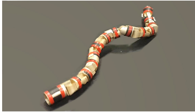
Figure 1. The snake-like robot is slithering forward. This snake-like robot is modular designed. Each joint axis is orthogonal to its neighbors with a rotation range of \pm 90^\circ .
