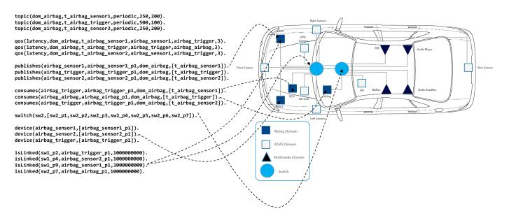
Fig. 1. An excerpt of the LP-based model of in-vehicle network using the formally defined facts. Using inference rules, interesting properties of the network can be verified.
