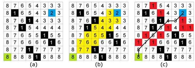
Fig. 2. Implementation of the Wavefront algorithm: (a) numeration of cells, (b) the set of intermediate points, and (c) the unfeasible points and the optimal path obtained by the Wavefront algorithm.
