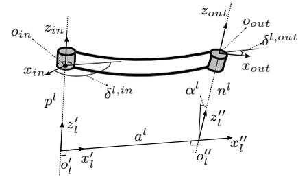
Fig. 2. Kinematic notation for link module characterization. The connectors are indicated in light-grey.
