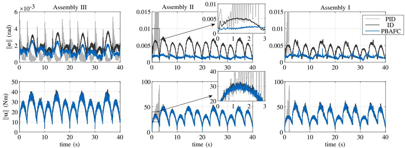
Fig. 8. Experimental comparison of different controllers for a changed assembly of the robot. We denote with ID the inverse dynamics control, with PBAFC the passivity-based control with adaptive friction compensation and with PID the scheme with decentralized PID controllers. PID control tests with assembly II and I had to be stopped due to instability.
