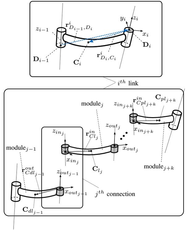
Fig. 4. Representation of a connection of modules that constitutes the  $i^{\text{th}}$  link of the manipulator involving parameters for dynamics. Connectors are indicated in light-grey.
