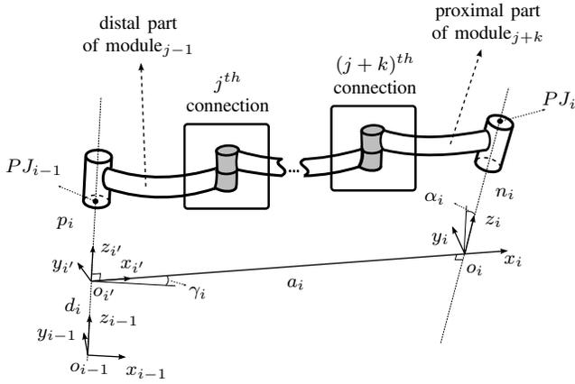
Fig. 3. Synthesis of kinematic parameters for the  $i^{\text{th}}$  constituted link with  $j$  being the cumulative number of modules connected.
