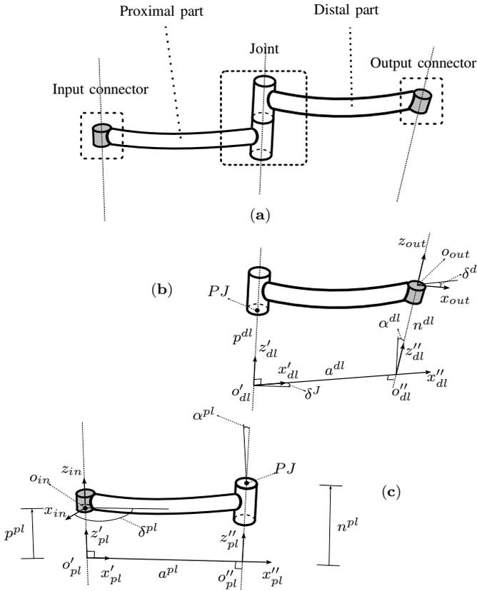
Fig. 1. Kinematic notation for joint module characterization. The connectors are indicated in light-grey. (a) is the entire module, (b) the distal part and (c) the proximal part.
