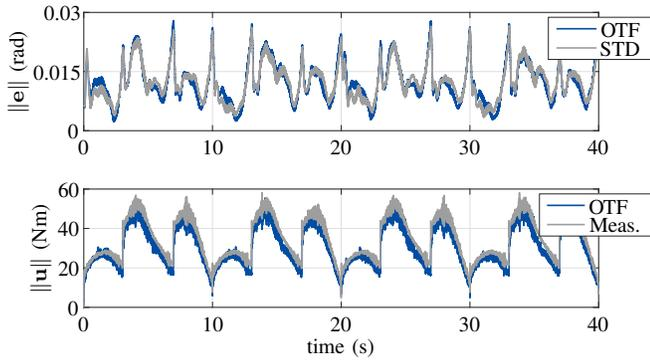
Fig. 6. Demonstration of the model accuracy. The first plot shows tracking performance of inverse dynamics control (with assembly I) using the model obtained with standard modelling approach (STD) and on-the-fly (OTF). In the second plot we show the matching between the measured torque for executing the motion and the prediction using the model generated on-the-fly.
