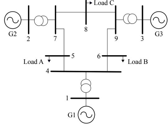
Fig. 3. The 3-machine 9-bus benchmark [18, Ch. 2].
