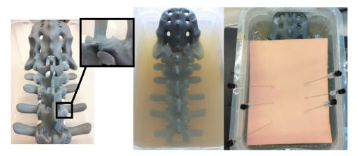
Fig. 5.18. Details on the phantom, (Left) Facet Joint simulated by silicone, (Center) Gelatin to simulate soft-tissue, (Right) Fabric cover to simulate skin
