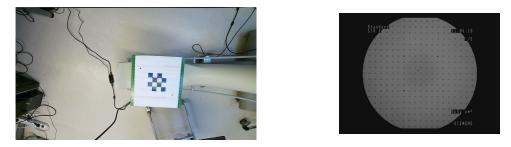
Fig. 5.7. Images of the checkerboard used by Wang et al. [173] in the (Left) video and the (Right) X-ray image
