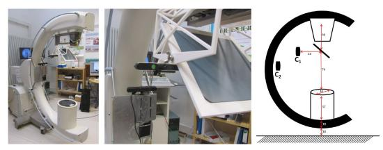
Fig. 7.1. (Left, Middle) The setup with the mirror-based RGBD augmented C-arm and an additional RGBD camera, (Right) The setup's sketch including the measured dimensions in centimeters
