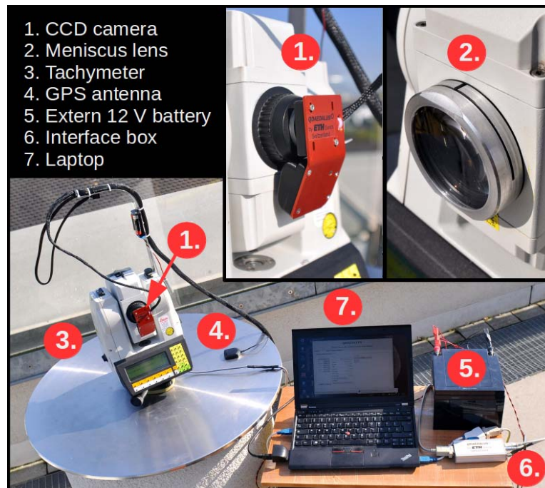
106 Fig. 1 QDaedalus system on the roof of the TUM. Note that the tachymeter shown is the Leica TDA5005, while 107 the results in this study are based on measurements with a Leica TCA2003.
