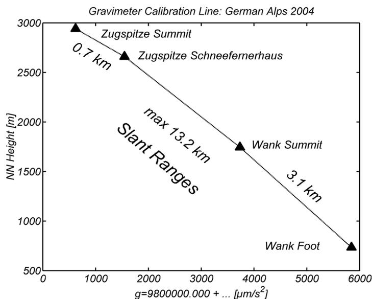
**Figure 4.** Distribution of the FG5-220 absolute gravity stations with respect to height and gravity range.
