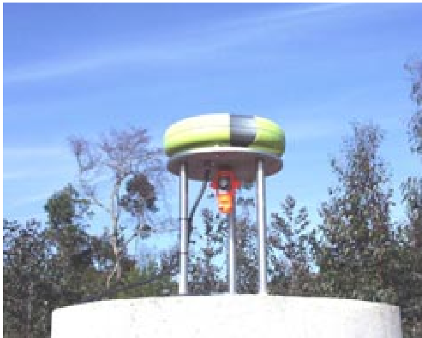
Figure 2: Survey pillar of the local network , Pillar with GPS/GLONASS antenna and reference point realized by the reflector
