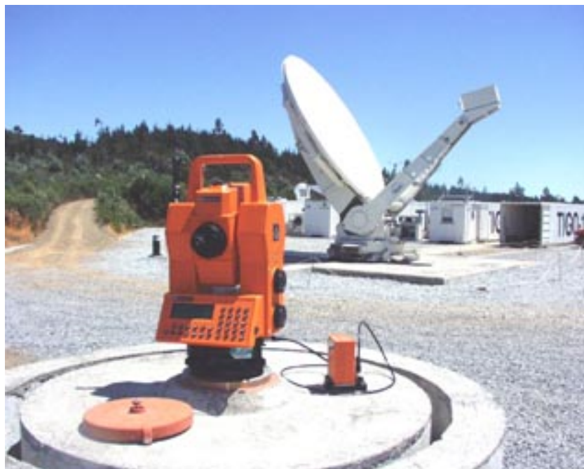
Figure 4: Tachymeter “Geodimeter Bergstrand” used for distance and direction observations
