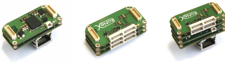
Figure 2.3: RoNex modules. Left: Base module — Middle: SPI module — Right: Both combined
