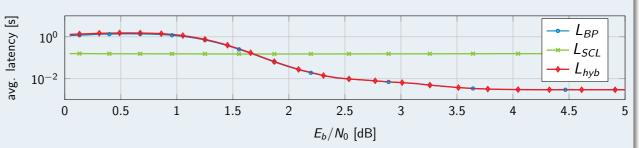
The maximum latency of the hybrid is lower bounded by the SCL-CRCs latency. For BP decoding the maximum latency depends on the maximum number of iterations.
