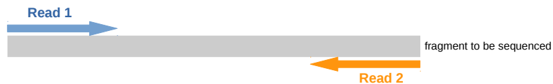
Figure 1.7.: Schematic illustration of the paired-end sequencing method where each fragment is sequenced from both ends. (Figure adapted from [89])
