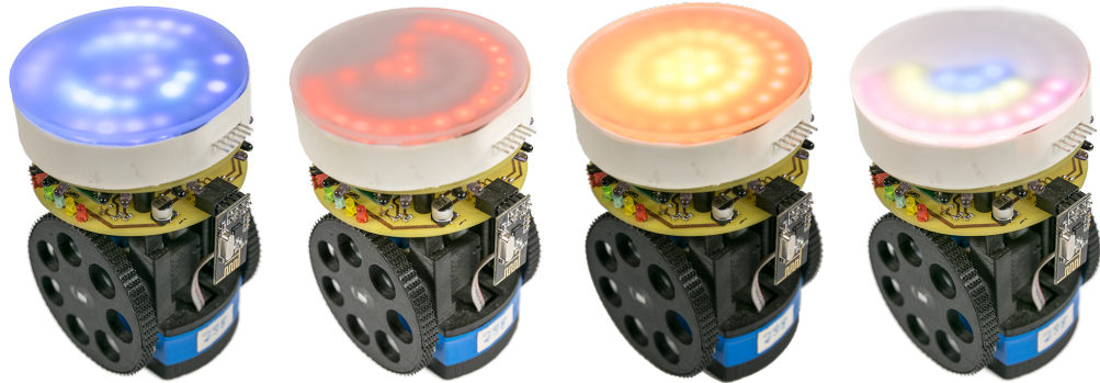
Figure 6.1.: A small two-wheeled robot which was developed at the Chair for Data Processing. The low-resolution led display on top is able to display basic emotions with dynamic light patterns (photographed by Martin Knopp).
