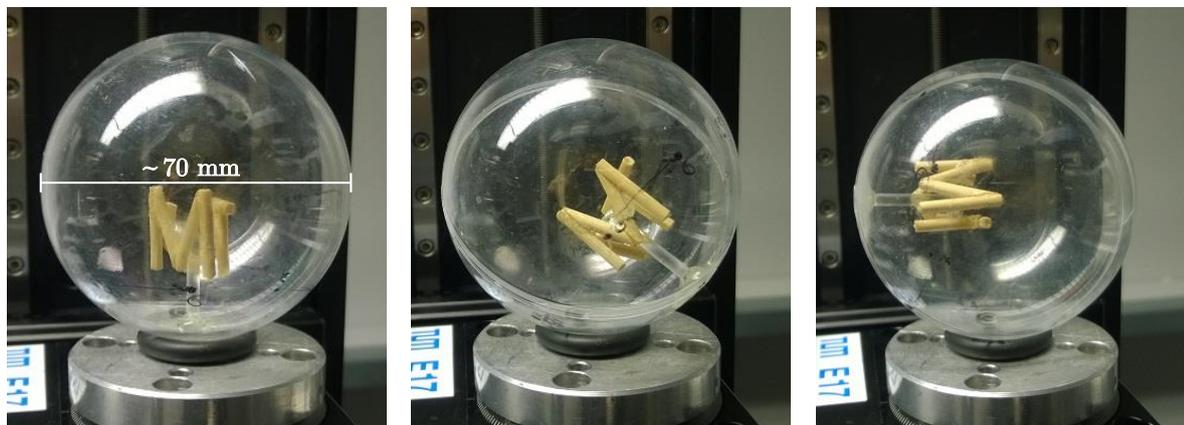
Figure 7.4: **Sample mounting for non-iterative directional dark-field tomography.** The sample is positioned inside a hollow sphere, which allows for an arbitrary positioning of the sample on top of the rotation stage.
