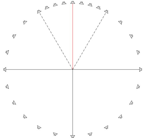
**Figure 1:** Loudspeaker setup for the localization experiment with a  $0^\circ$  head-above-torso orientation. The red line indicates the head position, the dashed lines indicate  $\pm 30^\circ$ .
