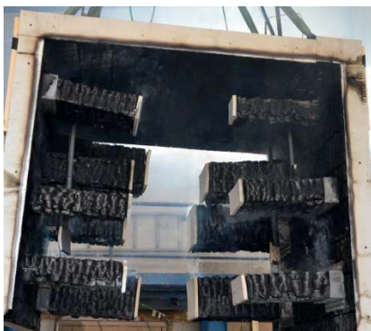
Figure 1. Unloaded test specimen after fire exposure.
