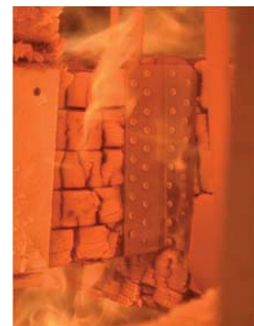
Figure 3. Loaded fire test with joist hanger.
