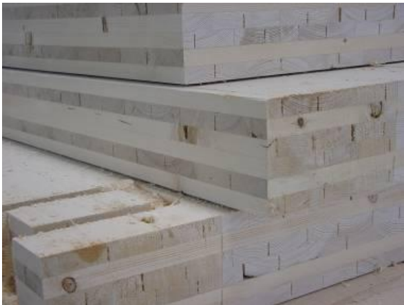
Figure 5: Cross laminated timber
