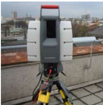
70. Full featured 360° 3D Laser-scanner on a tripod.
