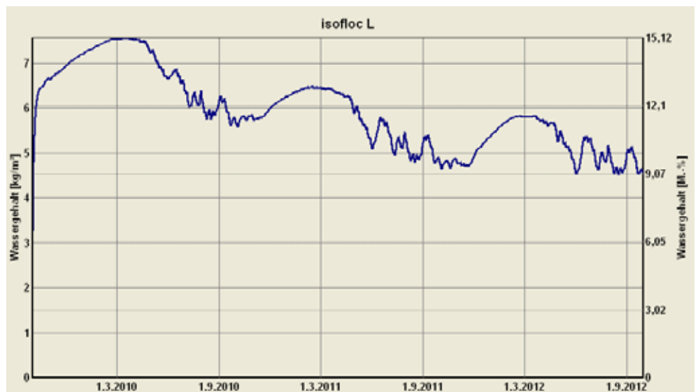
159. Humidity diagram of the cellulose fibre insulation layer shows the good drying capabilities during a range of three years. The overall mass of moisture in the element decreases.
