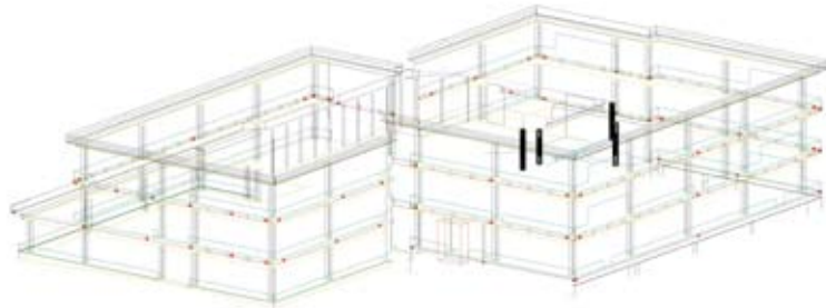
74. 3D wireframe model of the Realschule Buchloe was basis for the product model of the timber fabricator, surveyed in June 2009.
