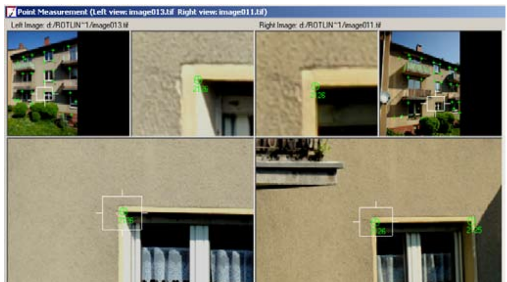
68. Multi-image 3D photogrammetry - postprocessing / 3D modeling of discreet façade points.
