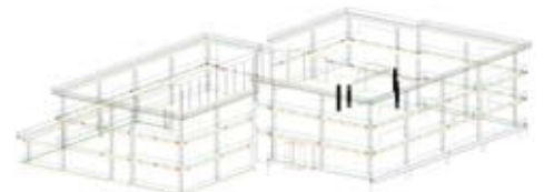
195. Survey result - 3D wireframe model of the main structure, ceilings and columns.
