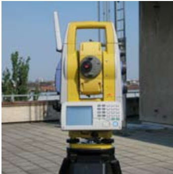
69. A modern Tacheometer also called Totalstation.
