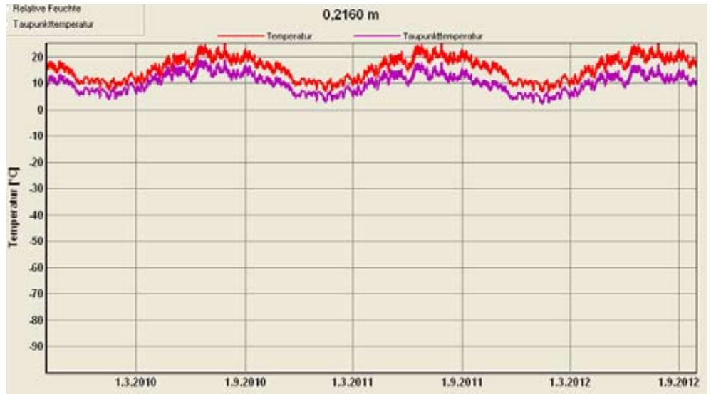
158. Temperature and dew-point diagram of the adaption layer during a range of three years. The red line indicates the temperature curve while the pink line shows the dew point temperature. The position is on the outside of the wood fibre hard board or the interior side of the TES element.
