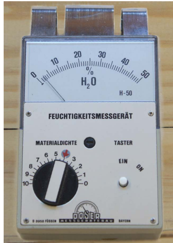
Fig. 12: Commercially available device using the capacitive method
