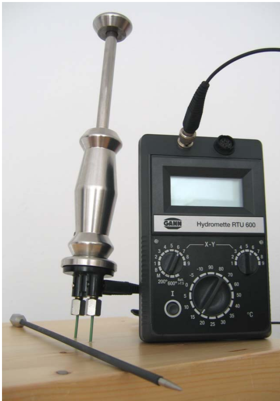
Fig. 11: Commercially available device using the resistance method
