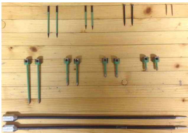
Fig. 13: Different types and lengths of insulated and non-insulated electrodes
