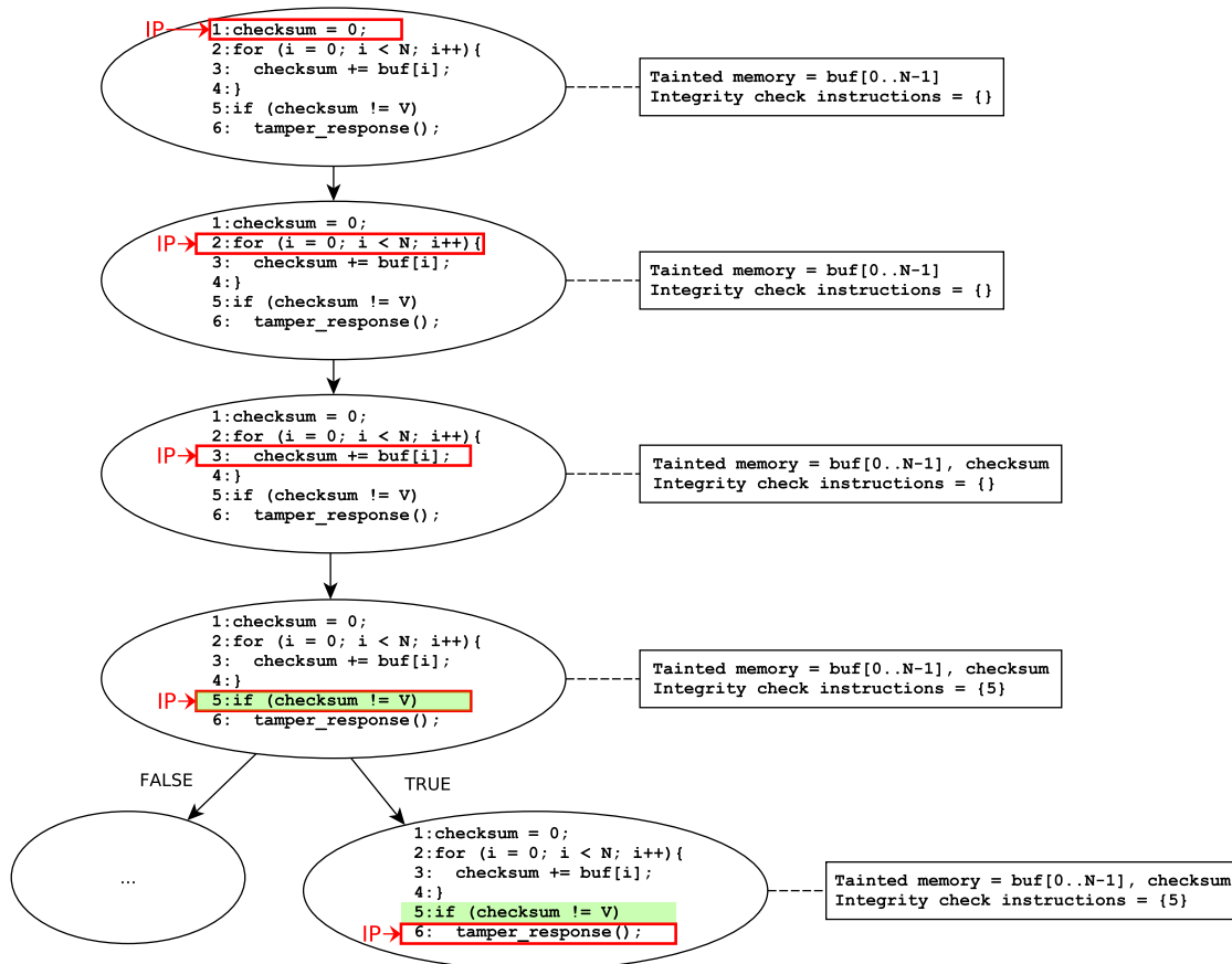
Figure 4.11.: Initial part of search tree corresponding to location recovery attack via taint analysis from Table 4.7.
