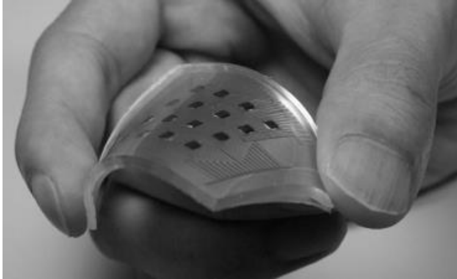
Figure 5.4: An example of 3D force sensor array based on the piezoresistive effect [208].
