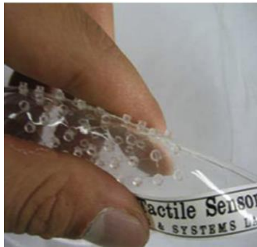
Figure 5.1: Fabricated prototype of optical fiber tactile sensors [202].
