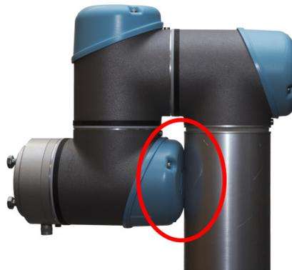
**Figure 5.4:** Close-up to the joint configuration of the UR5 showing a self collision.
