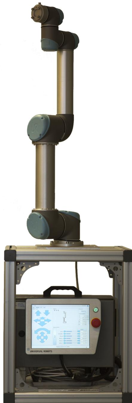
**Figure 5.3:** Universal Robots UR5, with a cart and control unit.
