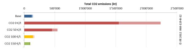
Figure 61: Total CO<sub>2</sub> emissions (kt) in CO<sub>2</sub> price scenarios in Europe (dark shading) and MENA (bright)
