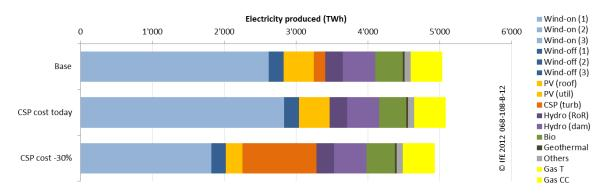
Figure 41: Electricity production by input commodity in CSP cost scenarios
