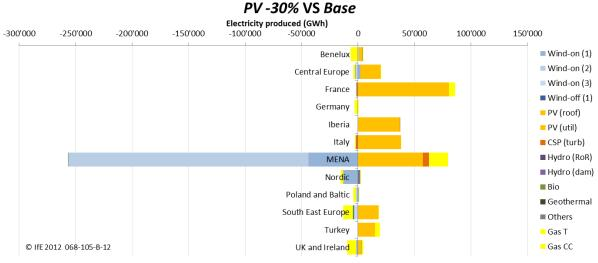
Figure 49: Difference of electricity production by region between scenario PV cost -30 % and Base
