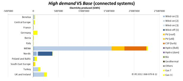
Figure 15: Difference in electricity production by region and input commodity between high and low demand (connected systems)
