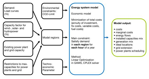
Figure 65: Overview of model input and output
