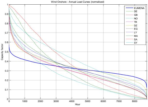
Figure 30: Standardized annual load curves of wind onshore capacity factors for EUMENA and 10 biggest contributors by installed capacity (scenario 01 *Base*).
