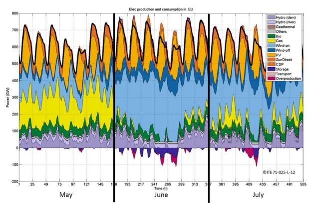
Figure 35: EU electricity production during three summer weeks in scenario 04 *Disconnected systems/High demand*.
