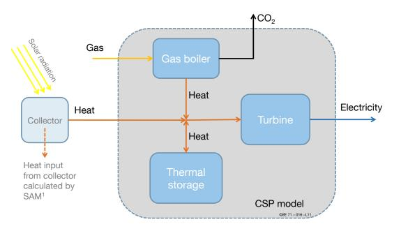
Figure 1: CSP model with its different components
