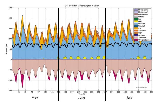
Figure 25: Electricity production time series with EU export (pale red) for MENA in scenario 01 Base.
