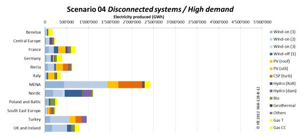
Figure 13: Electricity production by region and input commodity scenario 04 *Disconnected systems / High Demand*.
