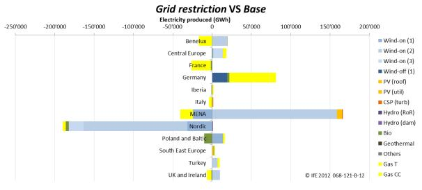
Figure 62: Difference of electricity production by region between s22 Grid restriction and s01 Base
