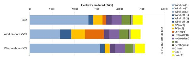
Figure 45: Electricity production by input commodity in wind onshore cost scenarios
