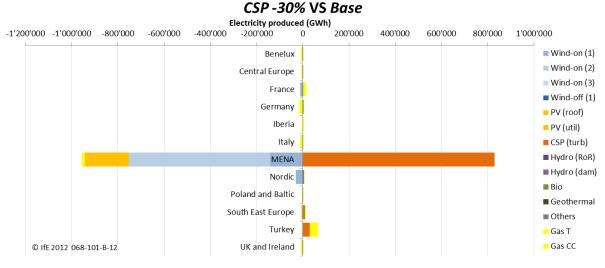
Figure 42: Difference in electricity production by region and input commodity between scenarios CSP cost -30 % and Base
