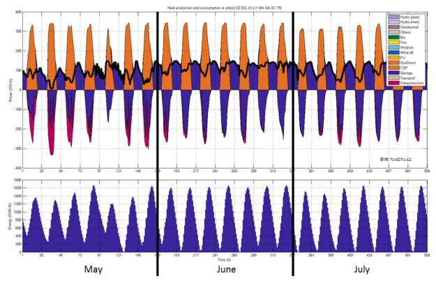
Figure 24: MENA use of CSP heat conversion (top) and storage (bottom) in scenario 03 *Disconnected* systems.
