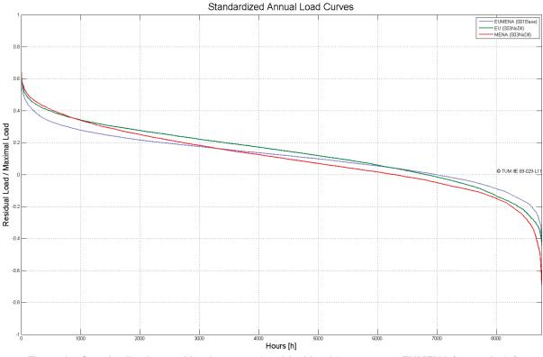
Figure 31: Standardized annual load curves of residual load for *connected* EUMENA (scenario 01) compared to *disconnected* EU & MENA (scenario 03).
