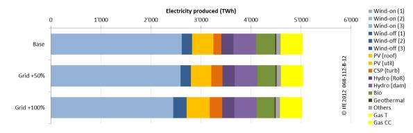
Figure 50: Electricity production by input commodity in grid cost scenarios
