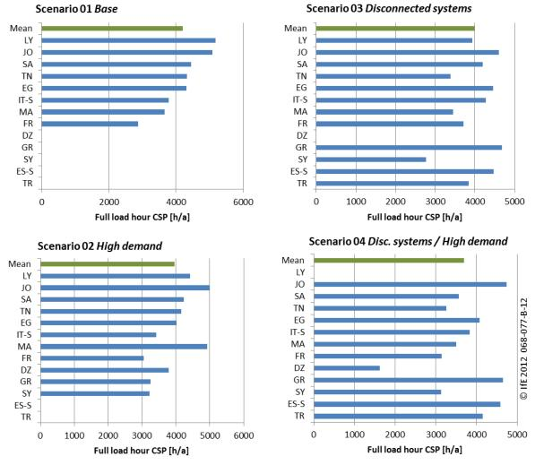
Figure 23: Full load hours of CSP for scenarios 01 to 04.
