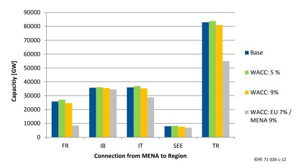
Figure 54: Installed transmission capacities between MENA and European regions for WACC scenarios
