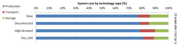
Figure 5: Relative shares of system costs by electricity generation, transmission and storage per scenario.
