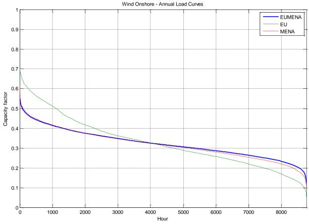
Figure 29: Standardized annual load curves of wind onshore capacity factors for connected EUMENA (scenario 01) and disconnected EU & MENA (scenario 03).
