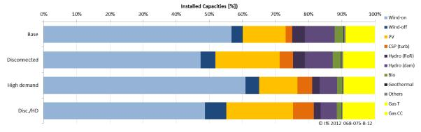
Figure 19: Relative shares of production capacities by input commodity and scenarios 01 to 04.
