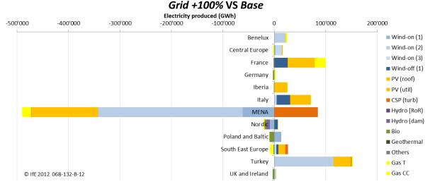
Figure 52: Difference of electricity production by region between scenario Grid cost +100 % and Base
