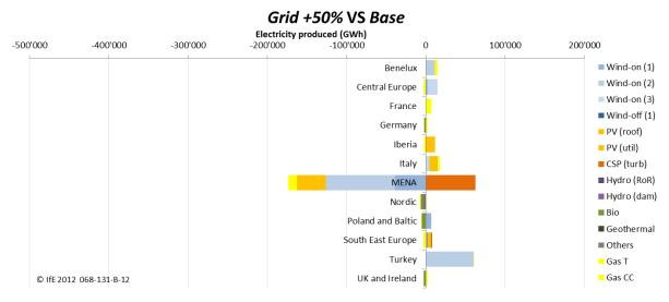
Figure 51: Difference of electricity production by region between scenario Grid cost +50 % and Base
