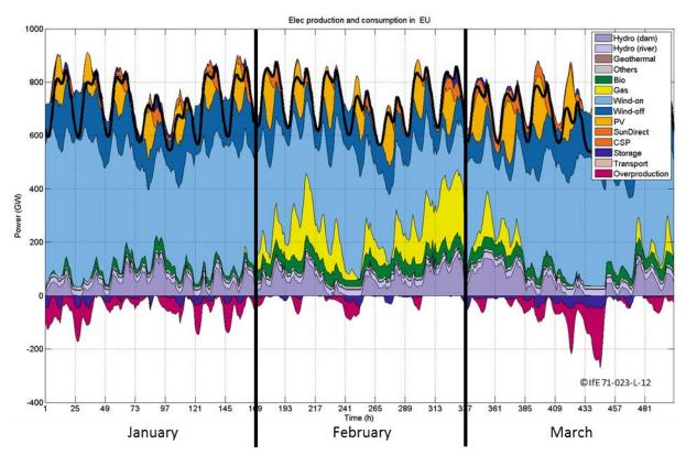
Figure 33: EU electricity production during three winter weeks in scenario 04 *High demand/Disconnected systems*.
