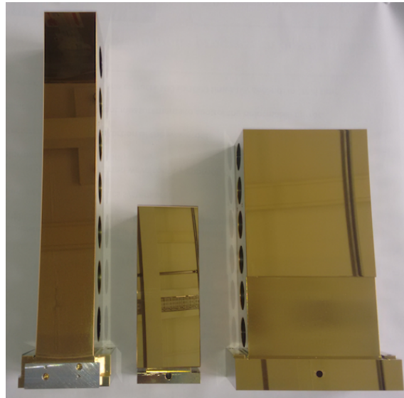
Figure 3.2.: The three mirrors of the SPIFFI spectrometer collimator. From left to right: M1, M2, M3
