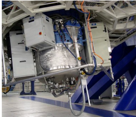
Figure 1.2.: SINFONI at the Cassegrain focus of VLT UT4. The aluminum vessel is the cryostat of SPIFFI and the blue upper part is the housing of MACAO. The grey boxes are the electrical cabinets.
