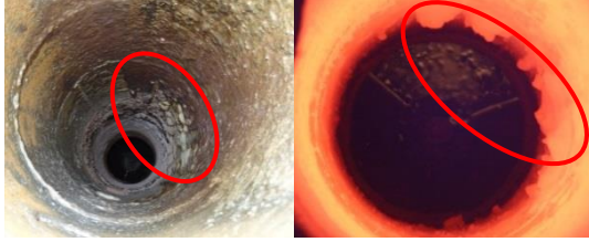
Figure 4: Slag on the wall in the cold (left) and in the hot (right) reaction chamber
