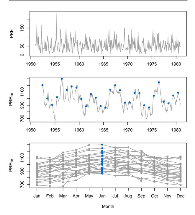
Figure 2.1: Illustration of Steps 1 and 2 of the computation of standardized drought indices in Section 2.1. The original precipitation (PRE) time series (upper panel) is aggregated at time scale  $\ell = 18$  (middle panel) and the 12 month-wise sub-series are extracted (lower panel). The blue dots correspond to the aggregated PRE<sub>18</sub> observations for June.
