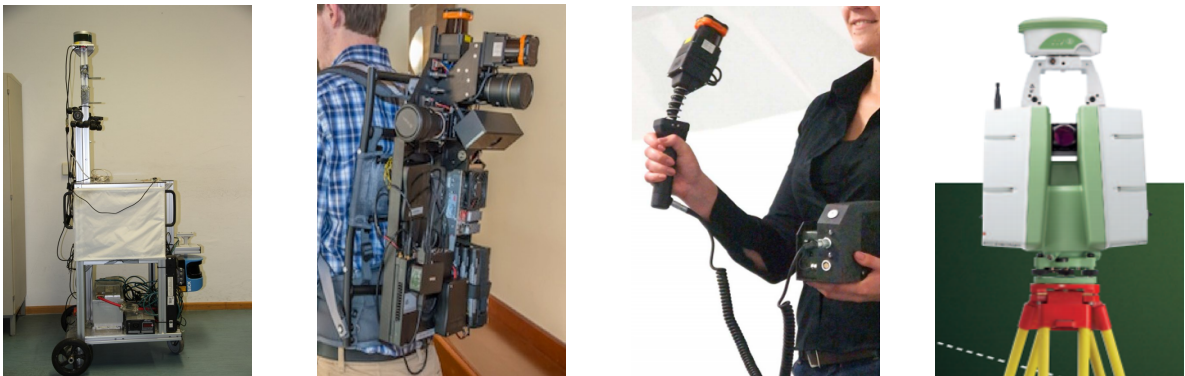
Figure 2.1: Four different types of LiDAR-based mappers. From left to right: LMT trolley-based mapper [18]; backpack-based mapper (image source: [22] – reproduced with permission); ZEB1 hand-held mapper (image source: [23] – reproduced under CC3.0); Leica static SCANSTATION C10 (image source: [24] – reproduced with permission).
