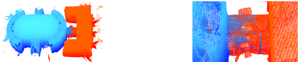
Figure 5.21: An example with extremely small overlap. The absence of salient features (objects with corners) means that no reliable CPSH can be computed even if appropriate segments are available. Image source: [2] – ©2016 Elsevier.
