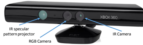
Figure 6.7: Kinect-like sensors emit a specular pattern using an IR projector whose reflection is captured by an IR camera. The projector-camera pair acts as a stereo camera used to recover the 3D shape of the surface on which the specular pattern is projected. The images returned by the RGB camera, which is calibrated w.r.t. the IR camera, can also be used to color the resulting point cloud.
