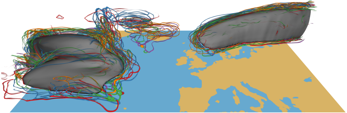
Figure 5.1: Visualization of a weather forecast ensemble from the ECMWF Prediction System [LP08]. This ensemble comprises wind velocity data and consists of 50 members. For one isovalue, all members are visualized as silhouettes of isosurfaces. Additionally, a mean ensemble member is rendered as a gray isosurface to enhance the visual perception of the spatial context. Color is used to cluster members by their similarity.
