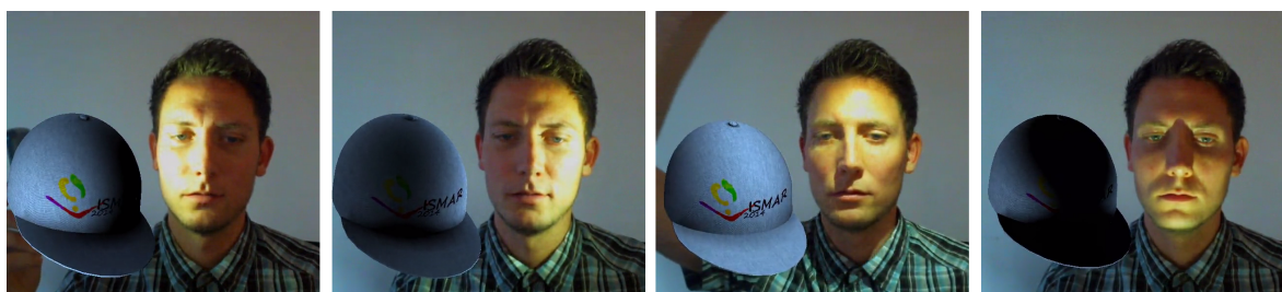
Figure 2.26: Examples showing a face under four different light directions and the coherent shading of a virtual cap. Note that the shading assumes that the virtual cap is positioned on the user's head – it has been moved and rotated for better visibility of the illuminated face.
