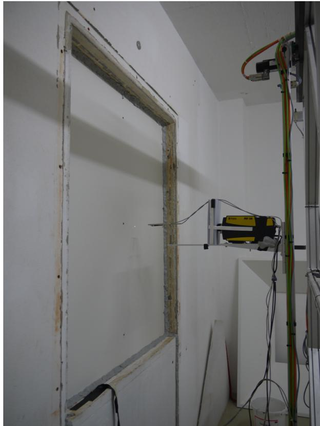
**Figure 4.3:** Aluminum plate with the intensity probe and the vibrometer [Angerer 2011] [Sremcevic Witzig 2012]
