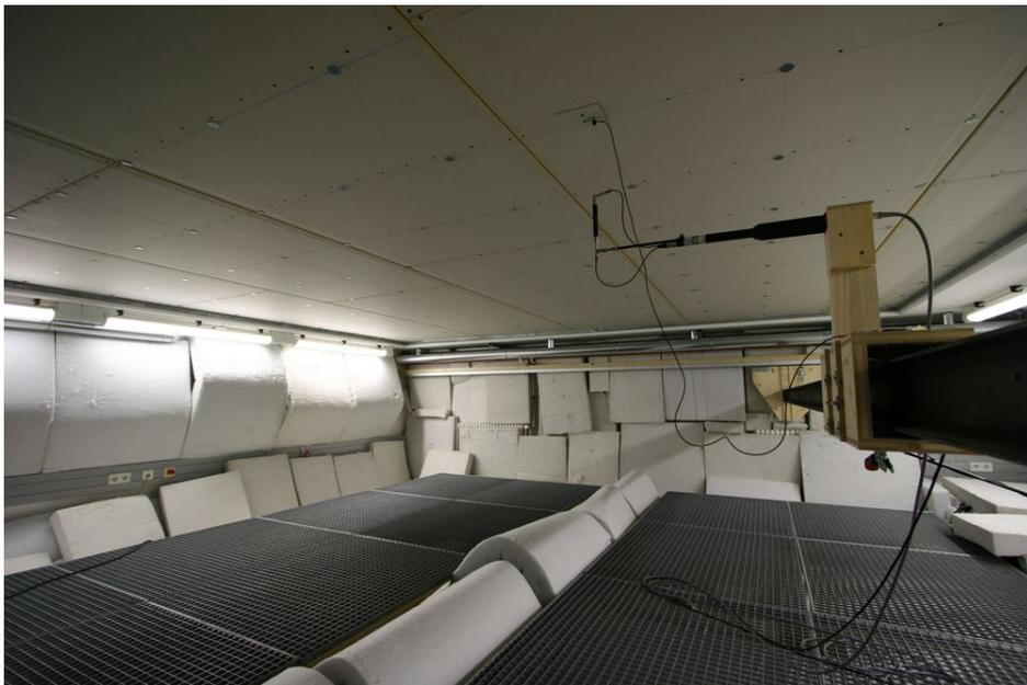
**Figure 1.3:** Simultaneous intensity and vibration measurement
