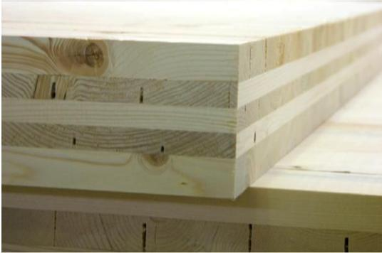
**Figure 3.6:** CLT cross-section
