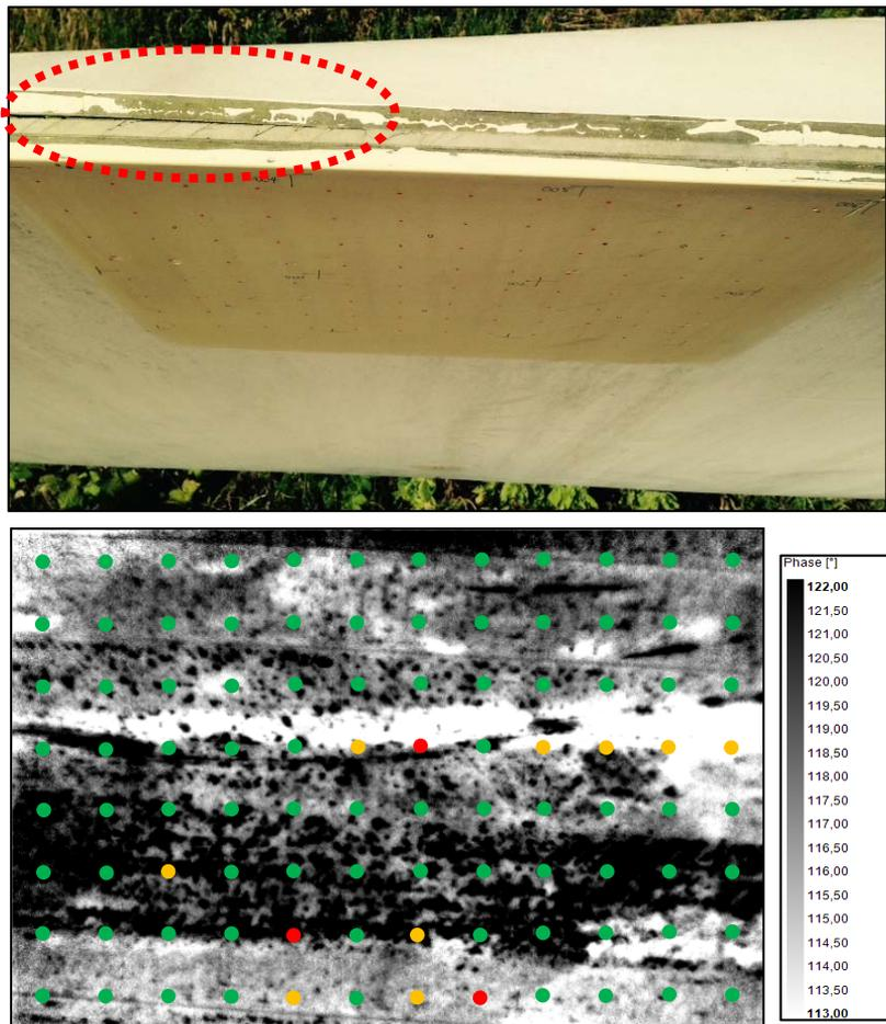
**Fig. 3:** Up: View of investigated trailing edge. Dashed encircled area: crack between bonding and shell located in the upper left corner of the tap area. Down: Results of an inspector’s rating comprising 8x12 tap points with 4 cm spacing. Green – intact, yellow – probably defective, and red – defective. Background: grey-scaled phase plot of modulated thermography method.
