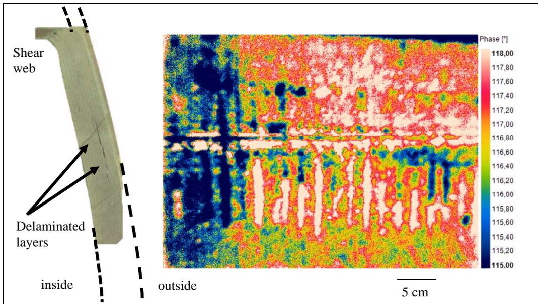
**Fig. 2:** Left: Cross section of spar cap (out of plane) featuring a delamination between material layers (arrows). Dashed lines indicate continuation of the cross section. Width of cross section: 4.8 cm. Right: Phase picture of modulated thermography measurement of roughly 30 cm height (in plane) and 40 cm width (out of plane).
