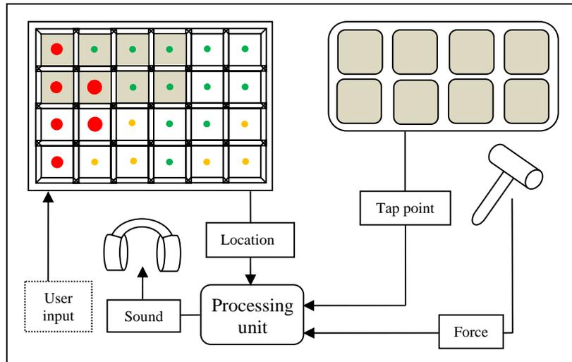
**Fig. 1:** General layout of the Tap Test Training System (TTTS). Upper left: User interface indicating active tap points, which can be tapped and edges for marking structural changes between tap points. Colored circles indicate ratings of the material integrity of the tap points. Upper right: Impact surface, here in the form of 8 discrete tap areas each representing one tap point of the recorded data. Processing unit combines all input data in real time and outputs the correct impact sound.
