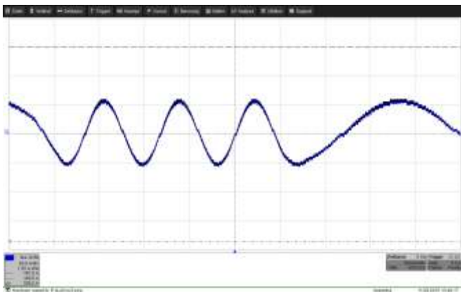
Fig. 13 – Measured stator current while reducing the sine frequency from 3 Hz to 2 Hz
