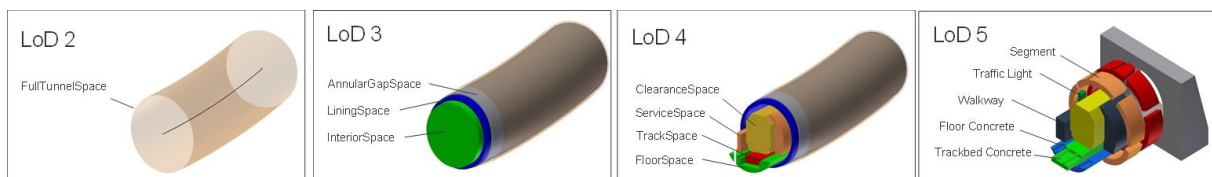
Figure 1: A 3D representation of the LoDs of the multi-scale shield tunnel product model (Borrmann and Jubierre, 2013). The first LoD, which only represents the alignment, is not depicted.
