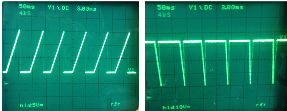
Figure 28: Left: scanner piezo voltage, right: sawtooth voltage applied to the base piezos.
