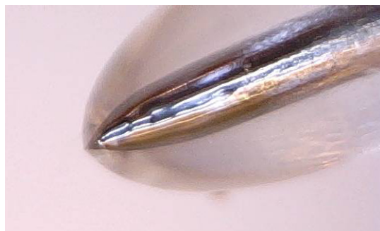
Figure 20: Etched tungsten tip coated with glue.
