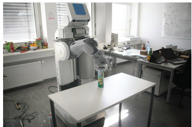
Fig. 22. Grasping of the localized object by the PR2 robot. The fitted geometric model was triangulated and fed into the grasp planning software to obtain grasping points.
