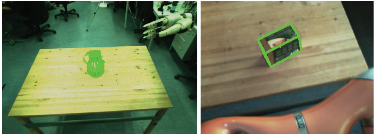
Fig. 24. Locating the resultant geometric model in an image by the TUM-Rosie robot.
