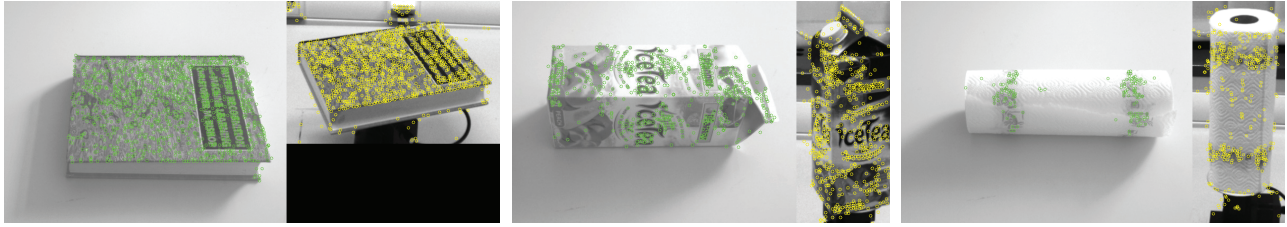
Fig. 13. Example of matching SIFT features for different objects from the imported database.
