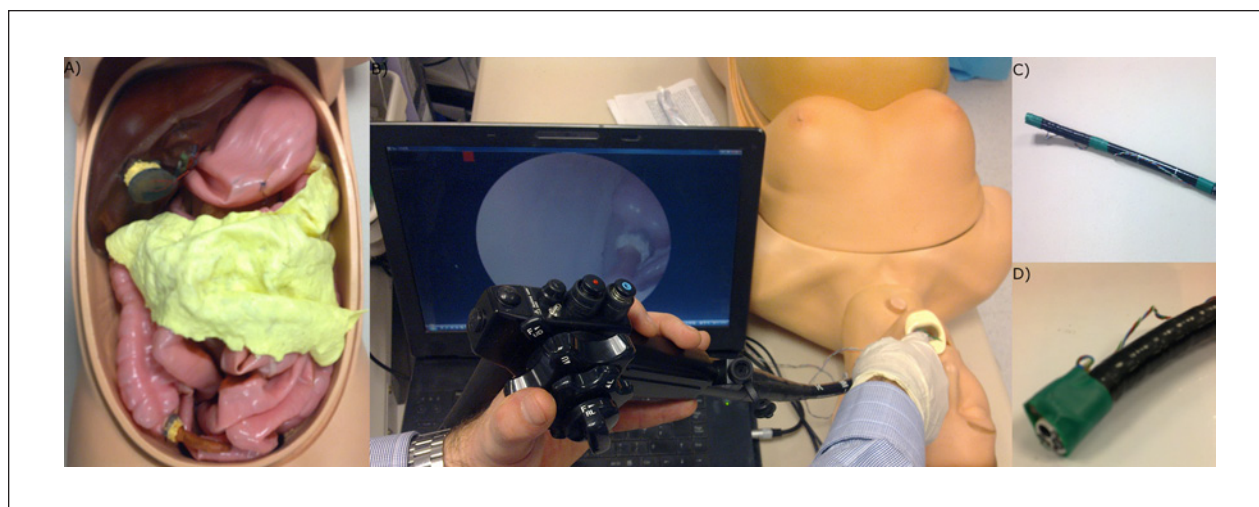
Figure 1. A. Overview of the abdominal components of the ELITE simulator with gastrostomy site visibly marked by sutures. B. Experimental setup with unaltered endoscopic view. Flexible endoscope with inertial measurement unit mounted at the tip (C and D).
