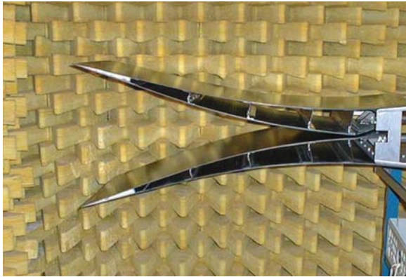
Fig. 11 Crocodile flap mode for yaw control and air brake function
