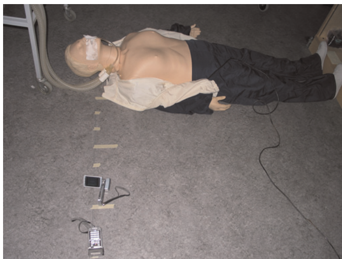
Figure 6 3G phone being used at ground level
