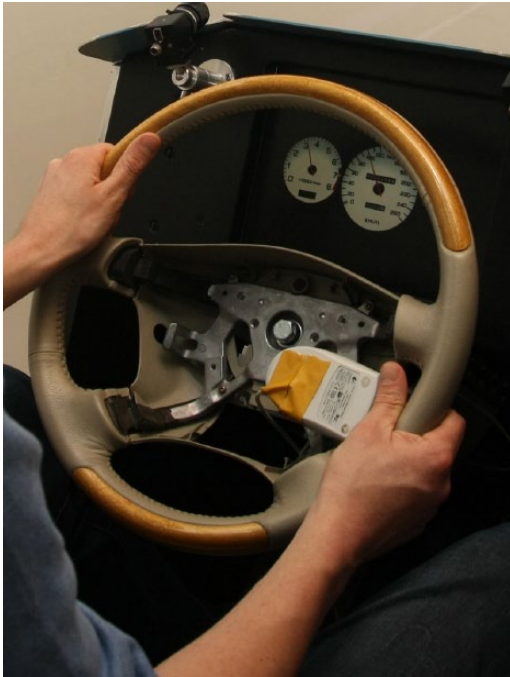
Figure 1. Close up of the steering wheel with the mouse attached.
