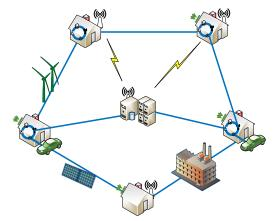
Since a typical power grid spans a large geographical area, the communication infrastructure plays a key role in the data delivery, and can potentially become a bottleneck. The delivery might be delayed, hence, making the data outdated, or it can be fully lost due to insufficient communication resources.
