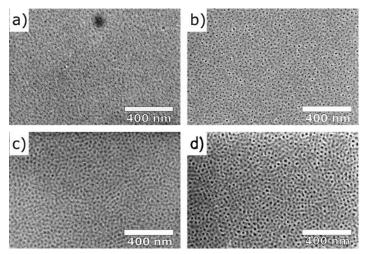
Figure 1: SEM image of nanoporous TiO2/SiO2 hybrid films with a 0.5 TiO<sub>2</sub>/SiO<sub>2</sub> ratio. The PS-*b*-PEO diblock copolymer was used as a template with a composition of a,b) 15.5-*b*-35.5 kg/mol and c,d) 20.5-*b*-8 kg/mol. a,c) before, b,d) after calcination at 400°C
