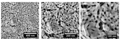
Figure 2: Mesoporous Ge layers for HPV applications
