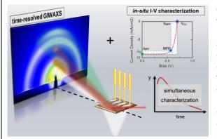
Figure 1: Schematic depiction of the setup of an *in-operando* GIWAXS experiment featuring simultaneous electronical and crystalline characterization
