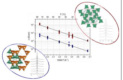
Figure 1: Temperature dependent Li ion conductivity (Arrhenius) determined by impedance spectroscopy, temperature dependence of <sup>7</sup>Li-NMR signal and structure of Li<sub>8</sub>SiP<sub>4</sub> (red) and Li<sub>2</sub>SiP<sub>2</sub> (blue).<sup>[1]</sup>
