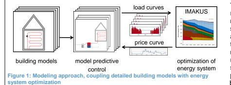
The German building stock is represented by detailed building models. These models are structured by building types and age. This approach allows scaling the heat demand of each building model according to the represented share of building space. During the investigated period, refurbishments and new building types change the building stock.
