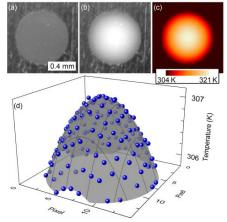
Figure 2: IR topography of suspended PEDOT:PSS a) without and b) under illumination. c) Temperature distribution under illumination. d) Exemplary fit (grey surface) of a measured temperature distribution (blue dots).
