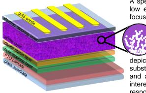
A special emphasis lies on environmentally friendly, cheap and low energy production routes. In that regard our approach is focusing on a completely water based hybrid solar cell. As
