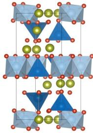
Figure 1: LTO crystal structure
