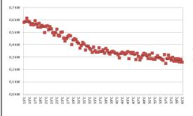
Figure 1: Thermal power output depends on return temperature (RT)
