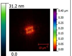
Figure 1: AFM image of imprinted active layer (left), 2 dimensional Fourier transformation of AFM image (right)
