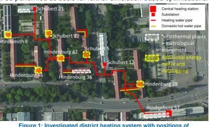
Figure 1: Investigated district heating system with positions of solarthermal plants
