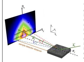
Figure 1. Schematic view of the GISAXS geometry: The incident angle of the incoming X-ray beam ( $k_i$ ) is  $\alpha_i$  and the exit angle of the scattered X-ray beam ( $k_f$ ) is  $\alpha_f$ . A beam stop is placed on the specular beam position.
