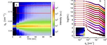
Figure 2. a) Full real-time mapping of horizontal cuts collected from in situ GISAXS data at  $q_z = 0.35 \text{ nm}^{-1}$ . b) Selected logarithmic plots of integrated horizontal cuts (solid dots), and fits (red solid lines). All the curves are shifted along the y-axis for clarity. The plots from bottom to top present the in situ time in a varied range from 2 s, 12 s, 18 s, 24 s, 30 s, 36 s, 42 s, 48 s, 54 s, 60 s, 66 s, 72 s, 78 s, and 96 s, respectively.
