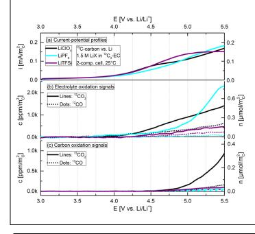
Figure 1: Carbon and electrolyte oxidation upon linear potential sweep from OCV to 5.5 V vs. Li/Li<sup>+</sup> at 0.1 mV/s with a <sup>13</sup>C-carbon working-electrode and a metallic lithium counter-electrode for an EC-based electrolyte with 1.5 M LiClO<sub>4</sub>, LiPF<sub>6</sub>, or LiTFSI respectively. (a): current-potential profile, (b): <sup>12</sup>CO/<sup>12</sup>CO<sub>2</sub> from electrolyte oxidation, (b): <sup>13</sup>CO/<sup>13</sup>CO<sub>2</sub> from carbon oxidation.
