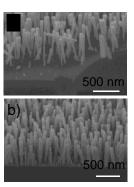
Fig. 3: Tilted-view SEM image of a) InN nanowires and of b) InGaN nanowires on Si (111).
