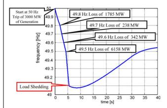
Figure 1: Frequency deviation after power plant outage [1]
