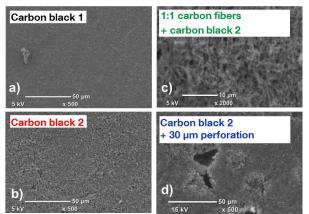
Figure 1: Scanning electron microscopy images of different microporous layer variations in top view.
