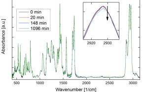
Figure 2: FT-IR absorption spectrum of active layer films measured at different illumination times, enlarged CH2 asymmetrical stretching peak
