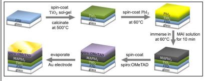
Figure 1: Solution conversion solar cell preparation routine
