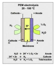
Figure 1: PEM water electrolysis.<sup>[1]</sup>
