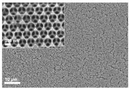
Figure 1: SEM micrograph of an obtained Ge film.
