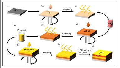
Figure 1: Fabrication process of the perovskite solar cell
