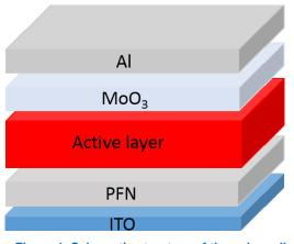
Figure 1. Schematic structure of the solar cell
