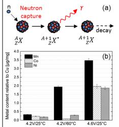
Figure 1: Neutron based Prompt Gamma Activation Analysis (PGAA) for quantitative and non-destructive detection of transition metal ions on graphite electrodes[1].
