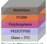
Figure 1: Bilayer stack of investigated solar cells.
