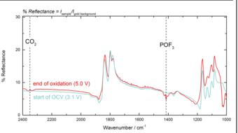
Figure 1: Operando DRIFTS data of an LFP half-cell with 1.5 M LiPF<sub>6</sub> in pure vinylene carbonate before and after oxidation to 5.0 V. The spectra show distinct signals of the gases  $CO_2$  and POF<sub>3</sub> after the oxidation process.
