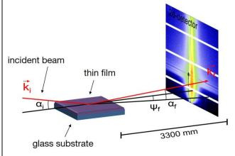
Figure 1: Schematic drawing of a GISAXS setup
