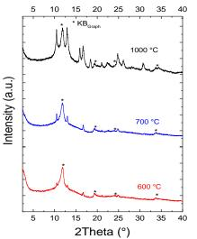
Figure 1: X-ray diffractograms of carbon supported Ta-based compounds synthesized at different temperatures
