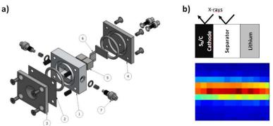
Figure 1: a) Exploded view of the spectro-electrochemical cell: (1) cell base; (2) X-ray window; (3) and (4) aluminum front-plate and back-plate; (5) stainless-steel current collectors; (6) electrode-separator assembly; (7) stainless-steel electric contact pins; b) Demonstration of spatial resolution; xray fluorescence mapping during open circuit voltage of the cell: sulfur signal ordered in S<sub>8</sub>-cathode
