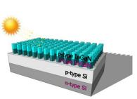
Fig. 2: Sketch of an InGaN nanowire/Si tandem solar cell.
