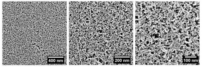
Fig. 1: SEM images of a mesoporous titania network at three different magnifications
