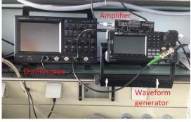
Figure 1: The setup for the MIS-Celiv including the oscilloscope, the wave form generator and the amplifier.
