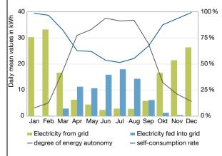
Figure 1: Self consumption and electricity exchange with the grid in the demonstration building
