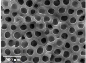
Figure 1. SEM of inverse opal structured Ge/Si
