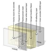
Fig. 2: Construction of the element / EBB
