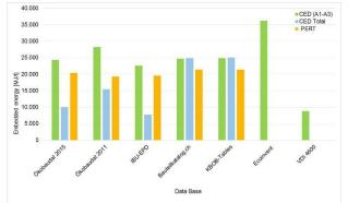
Figure 1: Embedded energy data for wood
