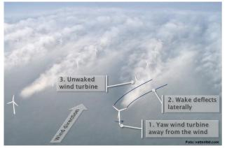
Figure 1: Concept of wind farm control by wake redirection
