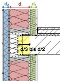
Figure 1: Connection detail wall-roof and its parameters
