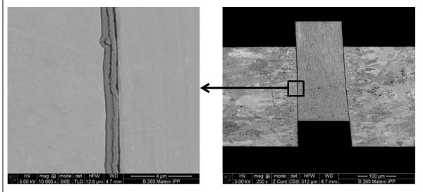
Figure 1: TiN as an interface Material after a Push Out test
