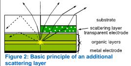
There are several approaches to increase the photon extraction which are based on adding scattering centers into the device. Besides the direct structuring of the substrate surface, the attachment of a transparent layer on the substrate is a very promising approach.
