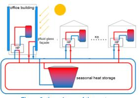
Figure 2: the scheme of the system
