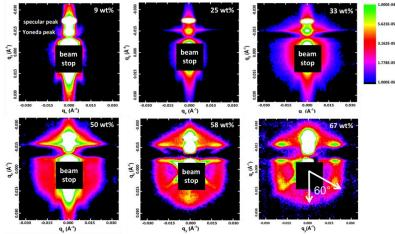
Figure 1. 2D GISANS patterns of P3HT-b-PS/PCBM bulk heterojunction system with 6 different PCBM weight fractions. Hexagonal orientation appears at a PCBM weight fraction of 67%.
