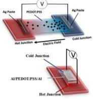
Figure 1: Schematic of in-plane(top) and cross-plane (bottom) Seebeck measurement setup
