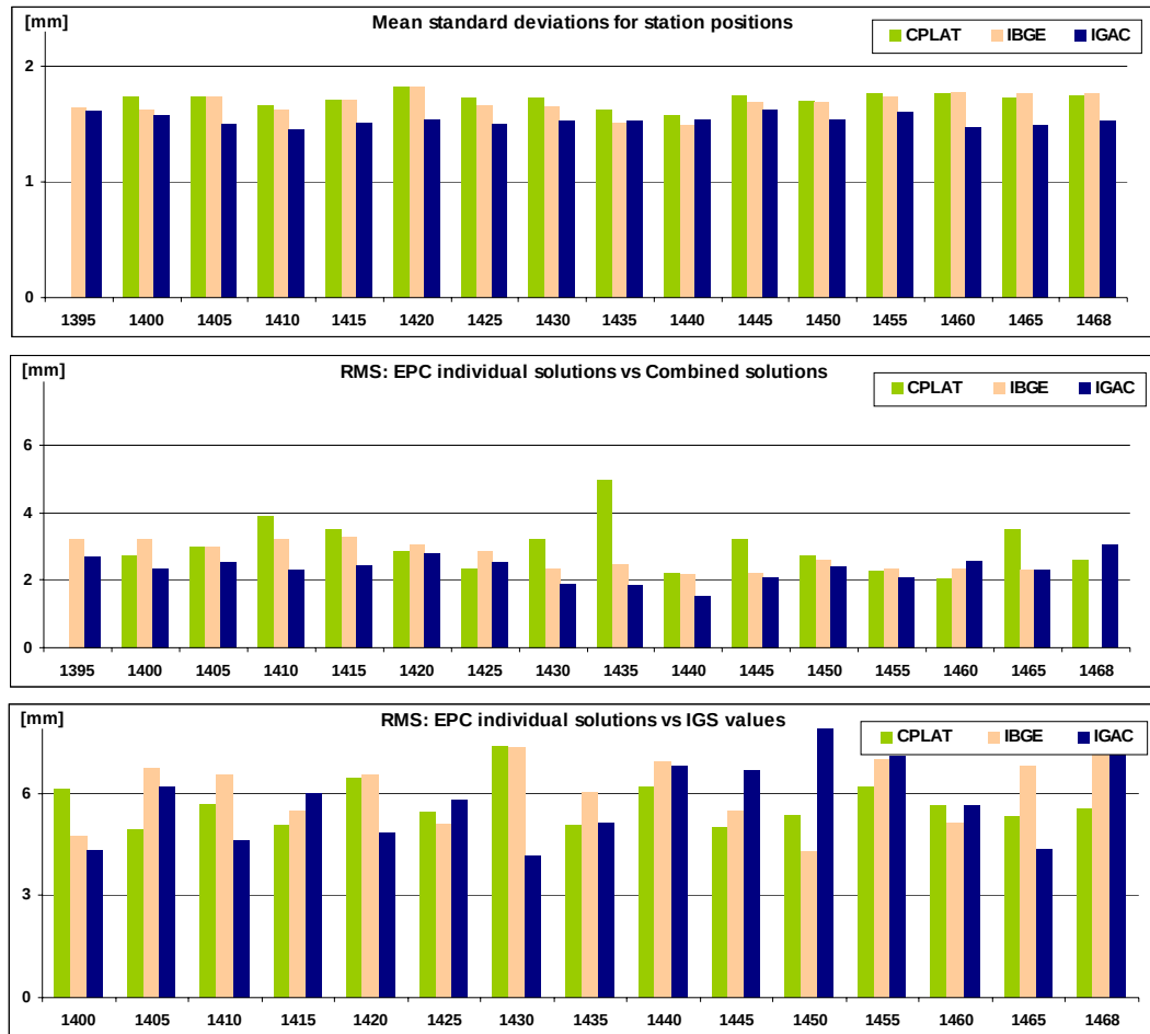
Figure 7. Mean standard deviations for the individual EPC solutions and RMS residuals between the EPC's weekly solutions and the combined solutions, as well as, with respect to the weekly IGS global network combination. (values for each fifth week are presented).
